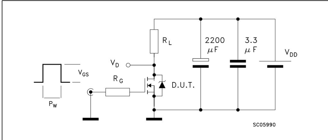
1. Max driver  $V_{GS}$  slope = 1V/ns (no DUT)
