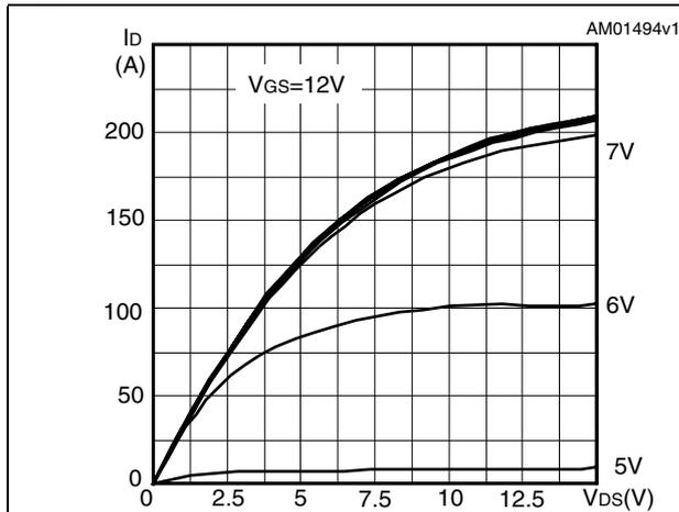
Figure 7. Transfer characteristics
