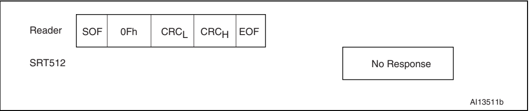
Figure 36. Completion frame exchange between reader and SRT512
