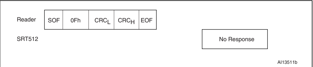
Figure 55. Completion frame exchange between reader and SRT512
