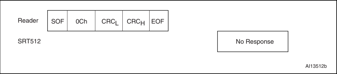
Figure 56. Reset_to_inventory frame exchange between reader and SRT512
