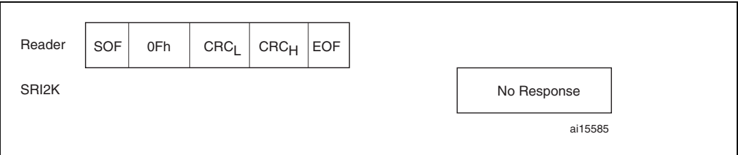
Figure 56. Completion frame exchange between reader and SRI2K
