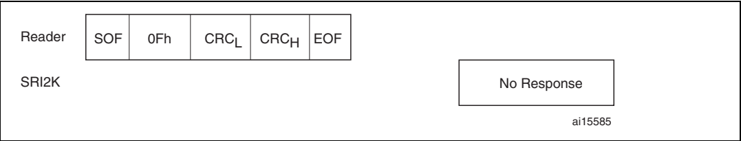
Figure 37. Completion frame exchange between reader and SRI2K
