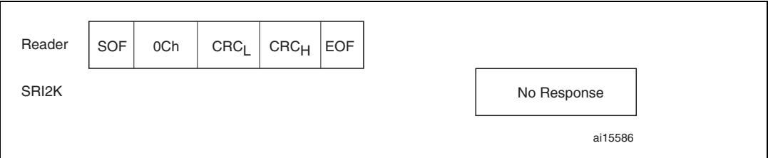
Figure 40. Reset_to_inventory frame exchange between reader and SRI2K
