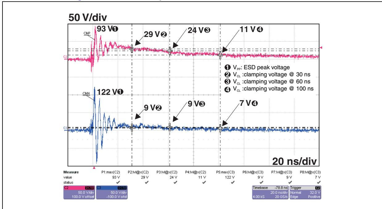
Figure 12. ESD response to IEC61000-4-2 (-8 kV contact discharge)
