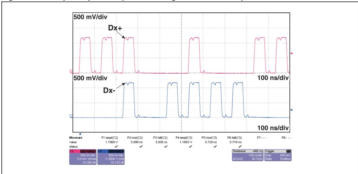
Figure 11. ESD response to IEC61000-4-2 (+8 kV contact discharge)
