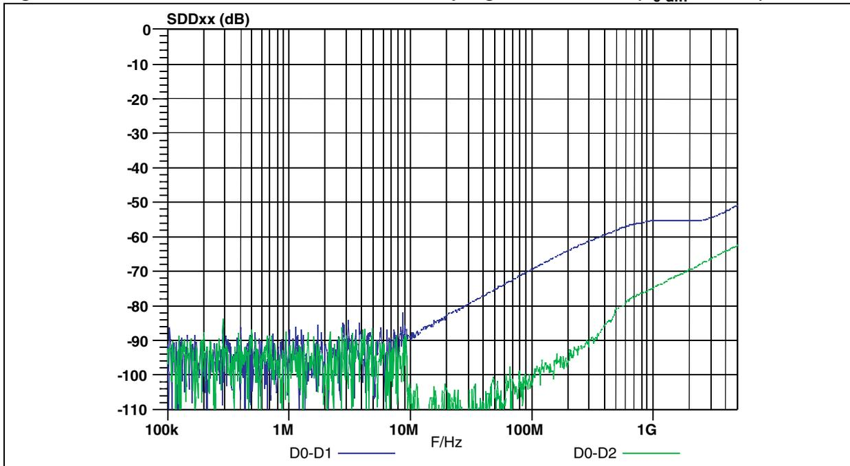
Figure 8. SCCXX inter-lane common-mode cross-coupling measurements ( $Z_{0\text{ diff}} = 100 \Omega$ )
