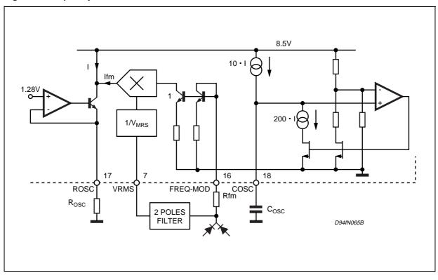
Figure 1. Frequency Modulation with L4981B.
