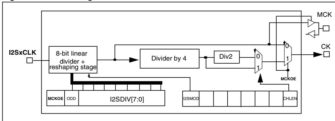
The audio sampling frequency may be 192 kHz, 96 kHz, 48 kHz, 44.1 kHz, 32 kHz, 22.05 kHz, 16 kHz, 11.025 kHz or 8 kHz. To reach the desired frequency, the linear divider (DIV) needs to be programmed according to the formulas below:
