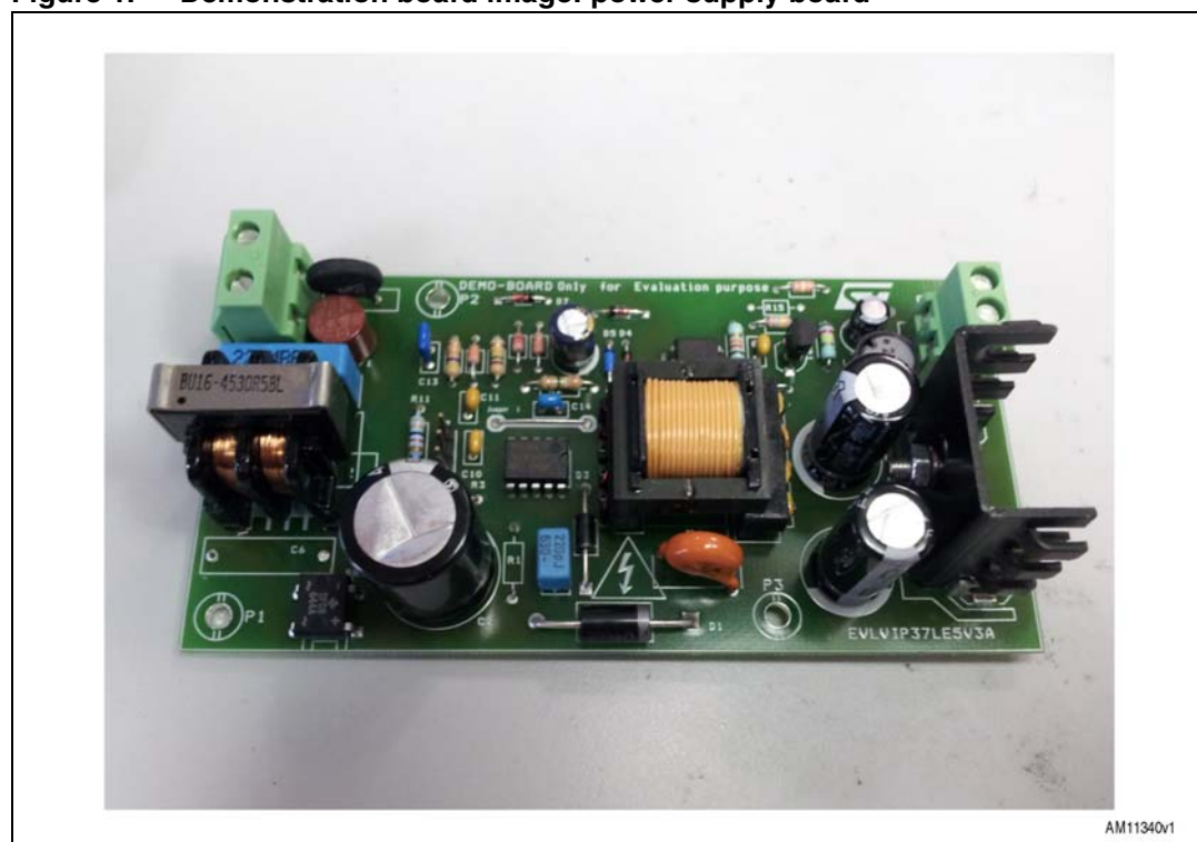
Figure 1. Demonstration board image: power supply board
