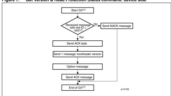
Figure 7. Get Version & Read Protection Status command: device side
