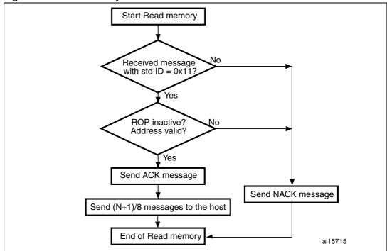
Figure 13. Read memory command: device side
