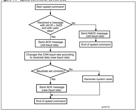
Figure 11. Speed command: device side
