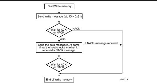
Note: If the start address is invalid, the command is NACKed by the device.
