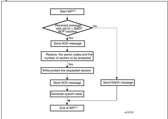
Figure 21. Write Protect command: device side
