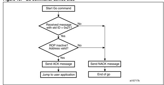
Figure 15. Go command: device side
