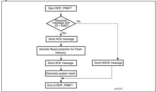
Figure 25. Readout Protect command: device side
