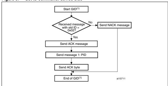
Figure 9. Get ID command: device side
