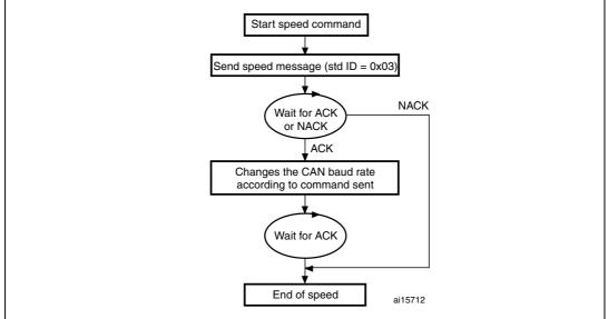
1. After setting the new baud rate, the bootloader sends the ACK message. Therefore, the host sets its baud rate while waiting for the ACK.
