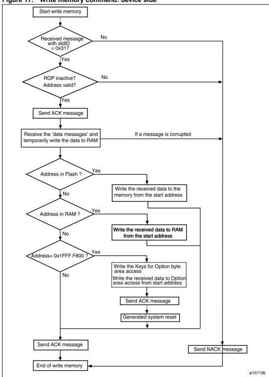
Figure 17. Write memory command: device side
