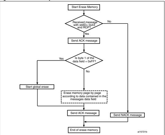
Figure 19. Erase Memory command: device side
