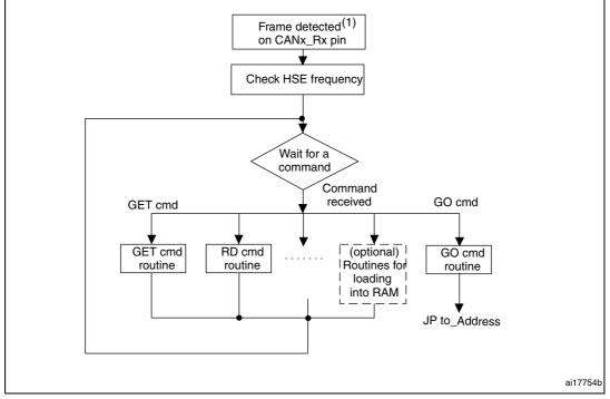
Figure 1. Bootloader for STM32 with CAN
