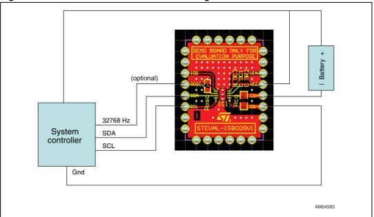
Figure 7. STC3100 demonstration board usage
