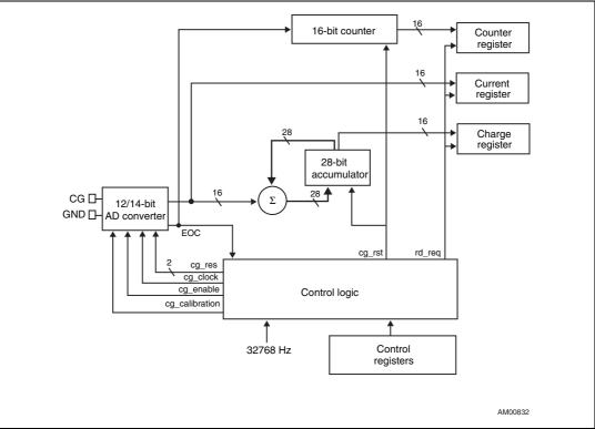
The A/D converter's output is a signed value in two's complement format. It is positive when the battery is charging and negative when the battery is discharging. When a conversion cycle is completed, the result is added to the charge accumulator and the 16-bit conversion counter is incremented.
