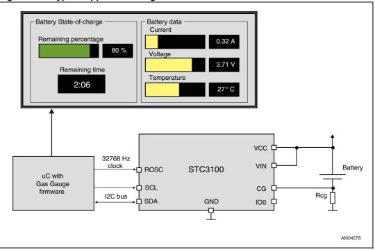
Figure 1. Typical application diagram for the STC3100
