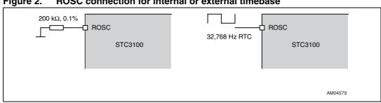
ROSC connection for internal or external timebase Figure 2.
