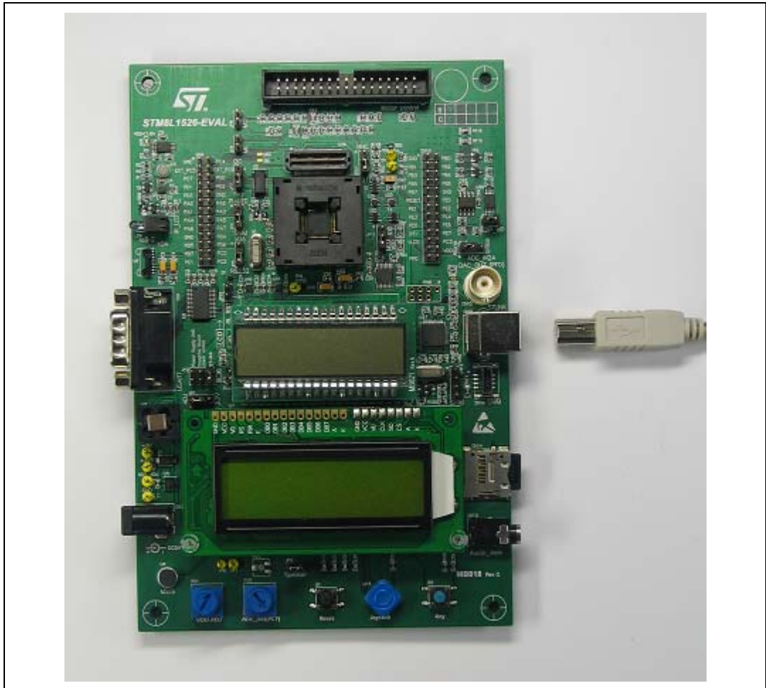
Figure 24. Connecting the debug instrument to the STM8L152x-EVAL evaluation board
