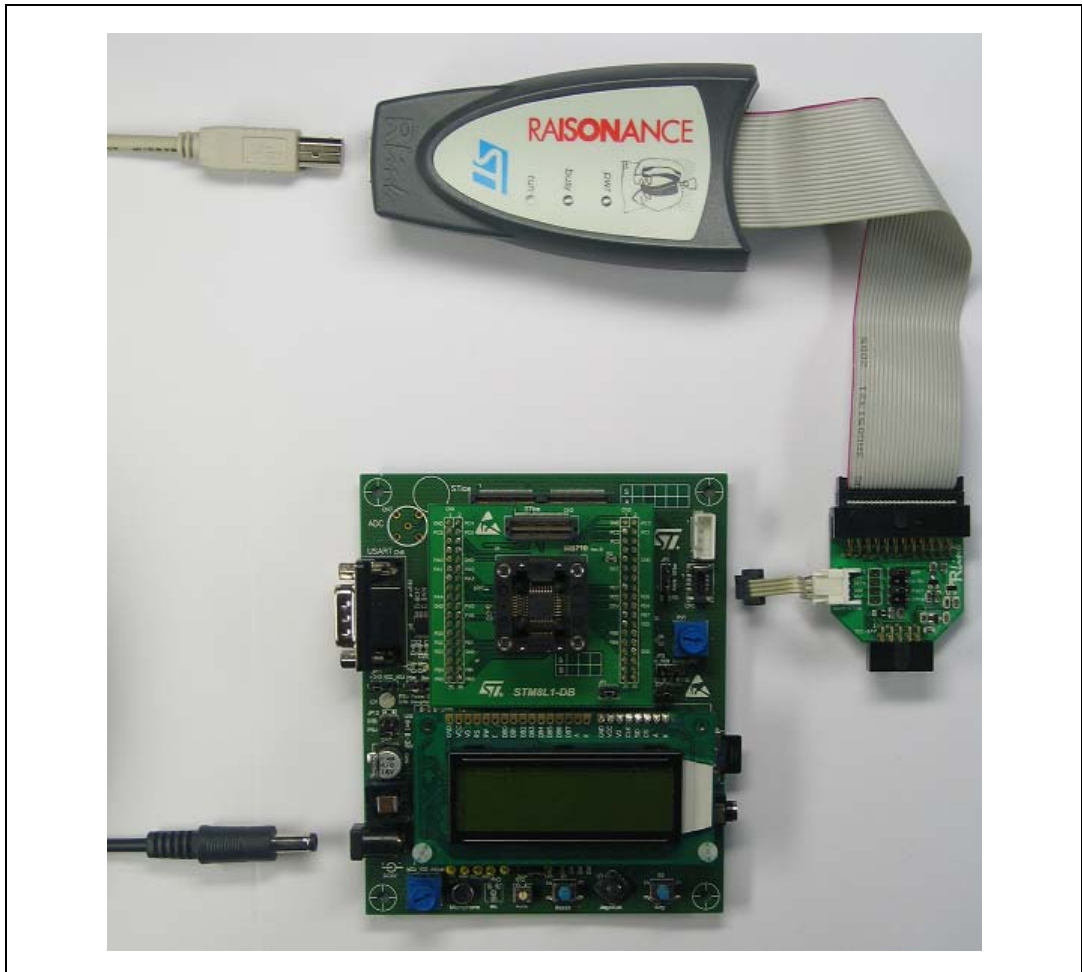
Figure 23. Connecting the debug instrument to the STM8L101-EVAL evaluation board
