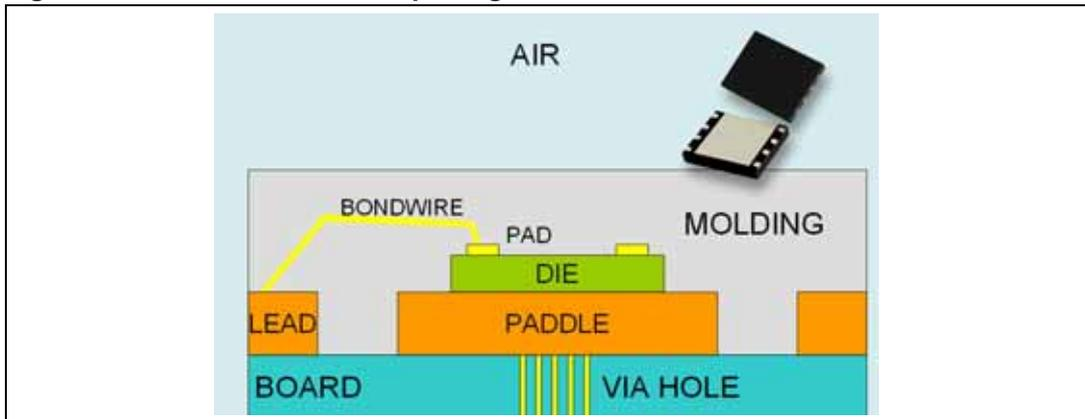
Figure 5. PowerFLAT cross-section
