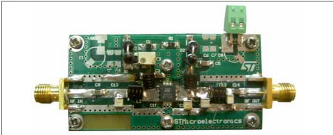
In the harmonic balance simulations we used all the information relative to the board and the S-parameters of the lumped capacitors and inductors. Figure 13 compares the simulations and measurements of the demonstration board at 155 MHz, varying the power delivered by the generator at the input port.
