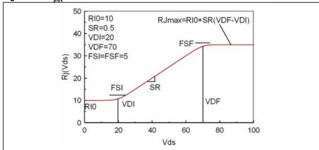
Useful to delete any convergence problem, [Figure 2](#) shows the resistor law for the variation of V<sub>ds</sub> (using the right hand function approach) ([Equation 13](#)). A similar graph and function can be obtained by varying V<sub>gs</sub> [3].
