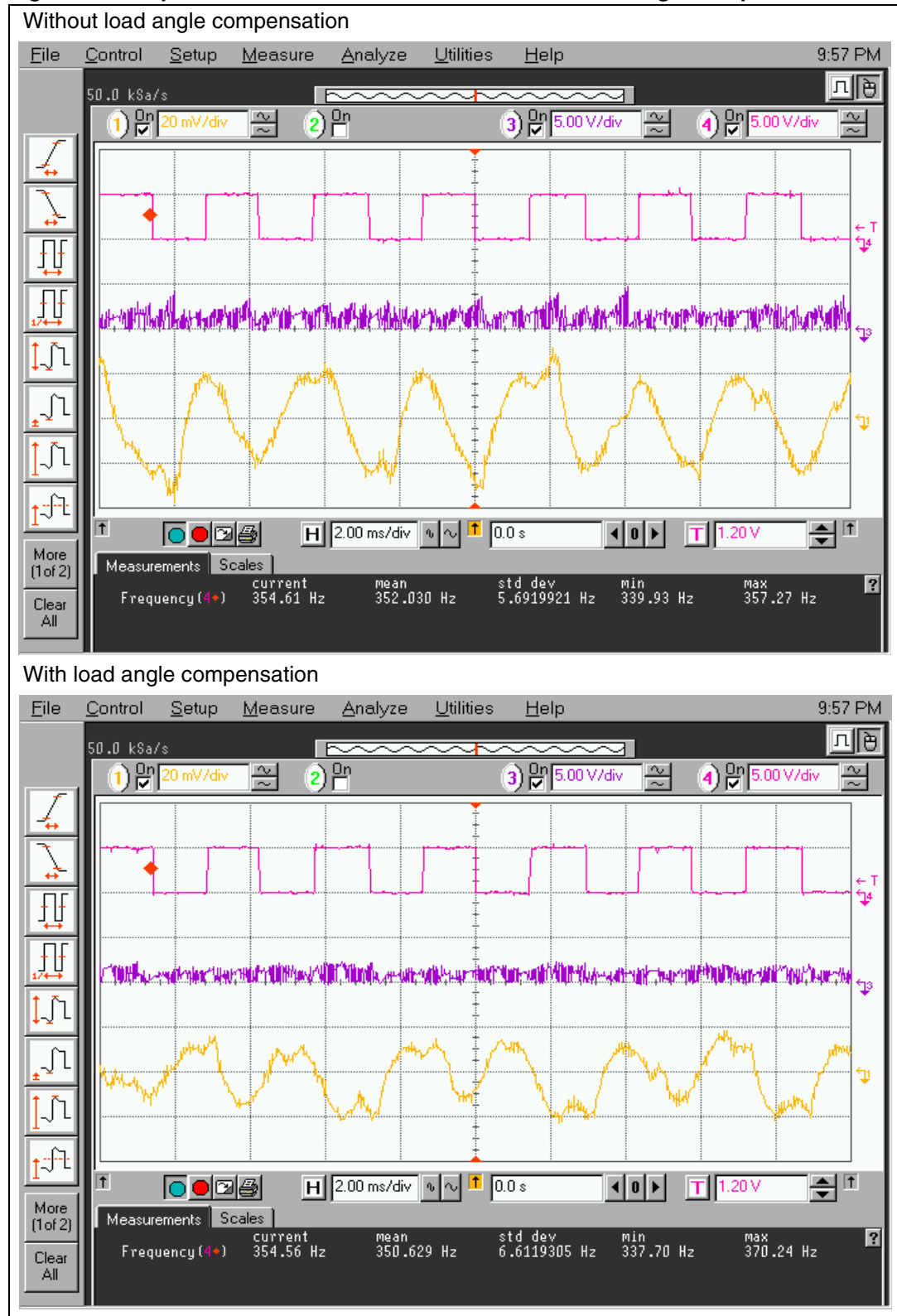
Figure 4. Experimental waveforms with and without load angle compensation
