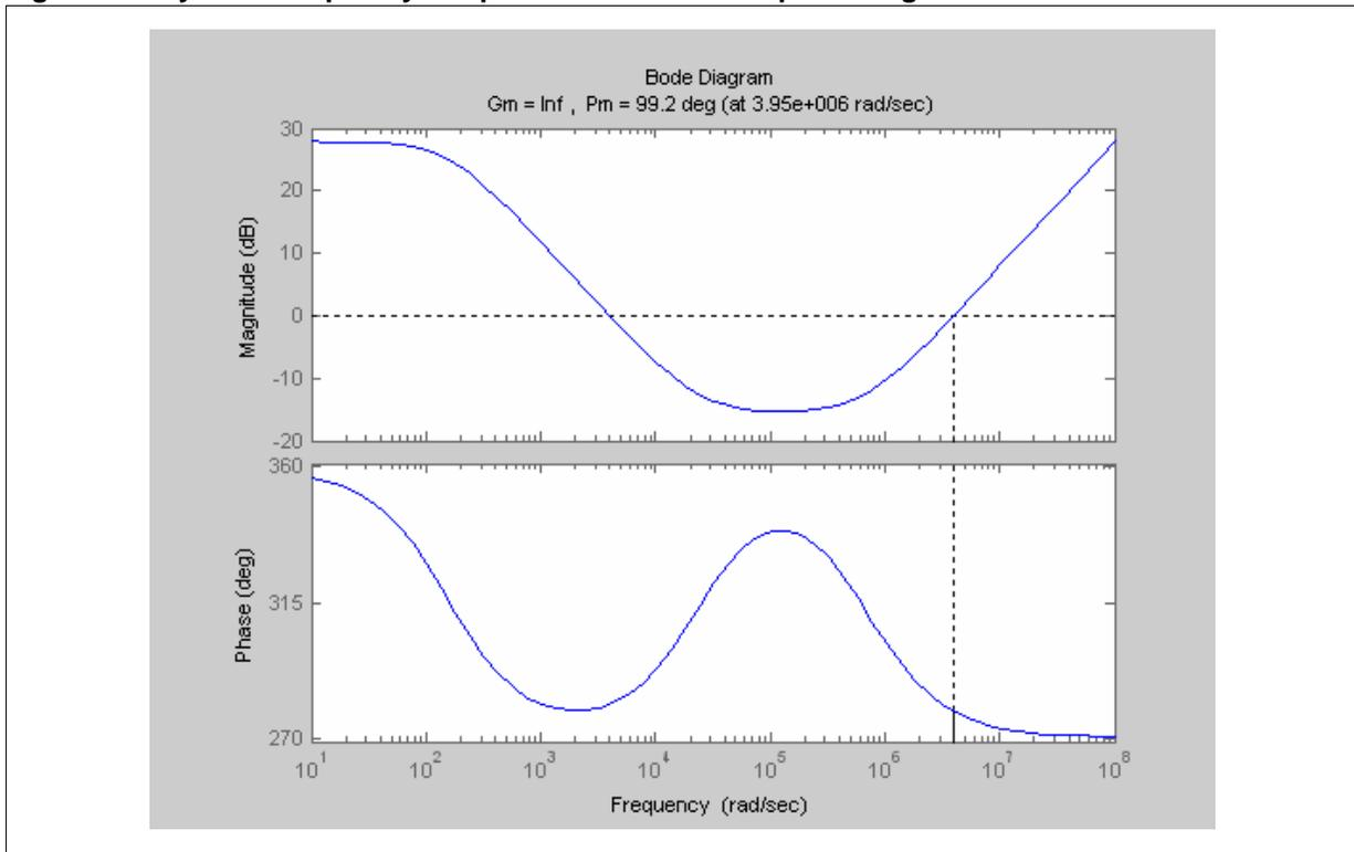
Figure 12. Stabilized Open Loop-transfer Function at Maximum Input Voltage
