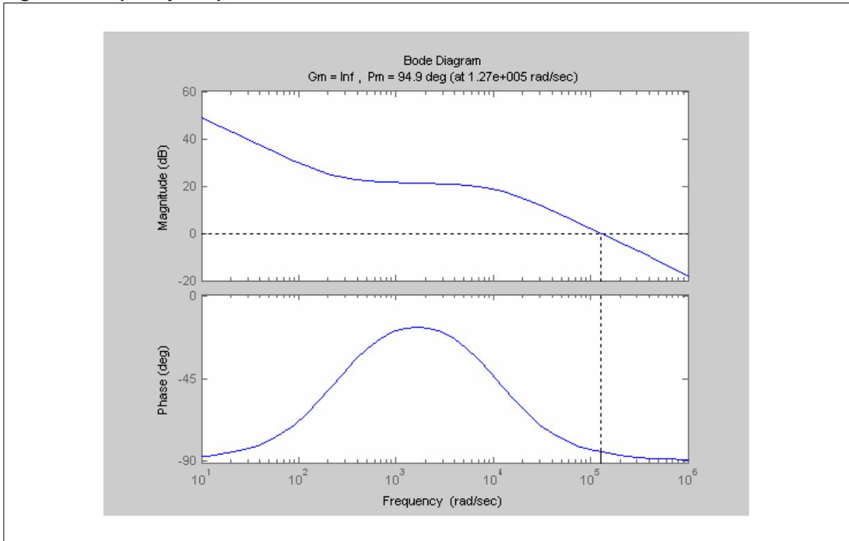
Figure 10. Stabilized Open Loop-transfer Function at Minimum Input Voltage
