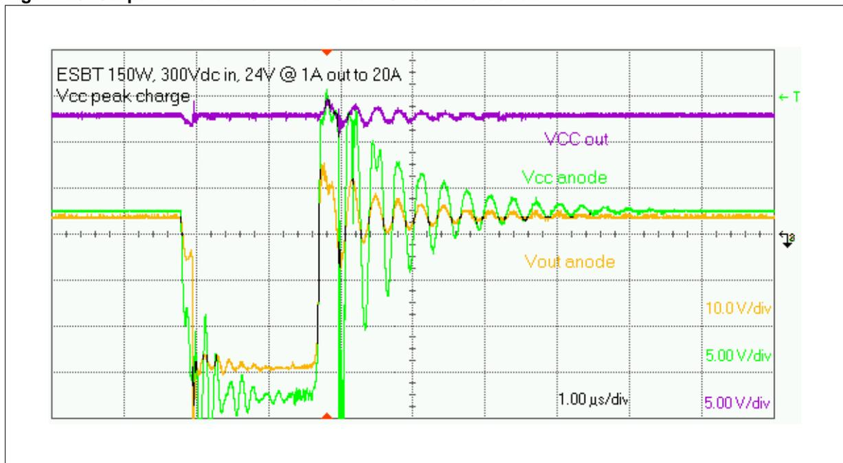
By adding a 22uH inductor in series with the Vcc winding and D3 we are able to filter out the spike and ringing to achieve Vcc to collapse below the under-voltage shutdown and re-initiate a start up. In this mode the high-cup mode is reached dissipating less power and keeping the thermal stresses low.
