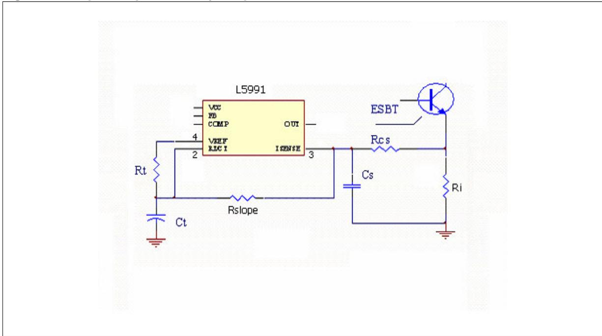
As seen in figure 18, a fraction of that voltage whose slope is  $\Delta V/\Delta t$  is added to  $V_i$  (the voltage across the current-sensing resistor). That slope is set at  $(N_s/N_p)R_i(m_2/2)$  by the  $R_{CS}$ ,  $R_{slope}$  resistors. Thus in figure 18, since  $R_i$  is much less than  $R_{CS}$ , the voltage delivered to the current sensing terminal (pin 13) is:
