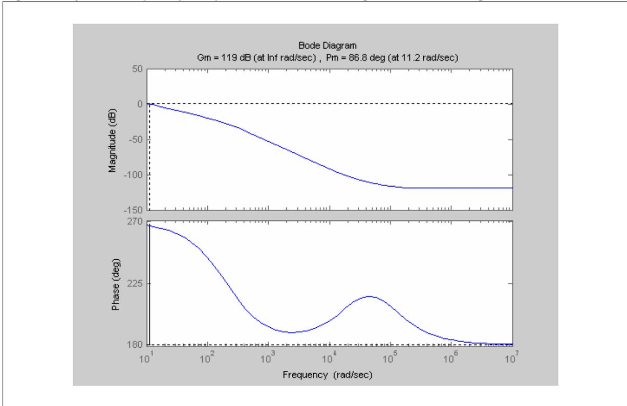
Figure 9. Frequency Response of the Feedback-transfer Function
