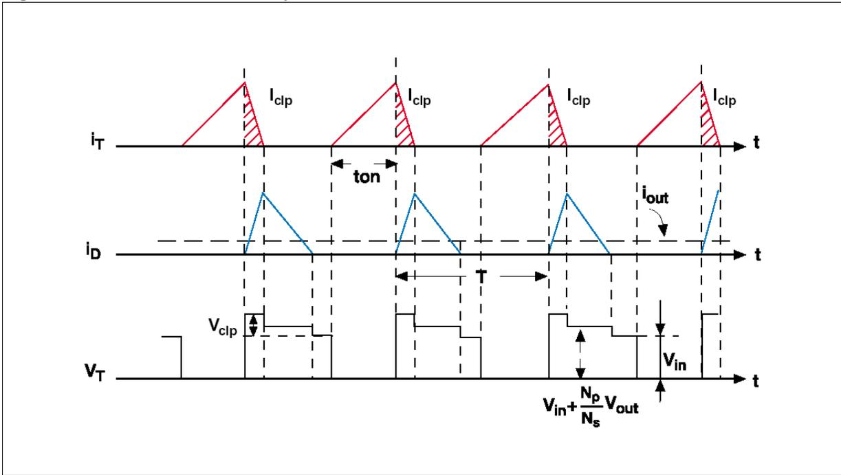
Figure 3. Continuous Mode Flyback Waveforms
