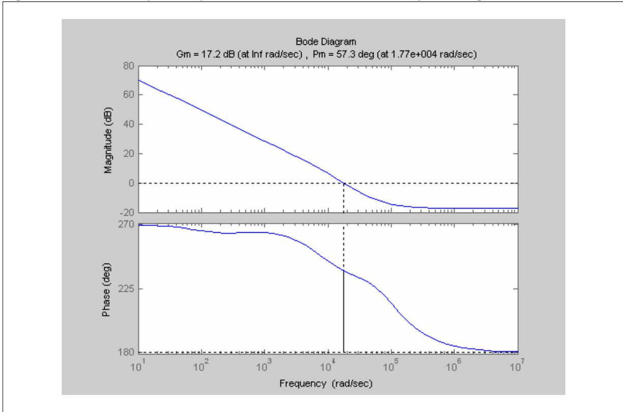
Figure 11. Flyback Frequency Response at Maximum Input Voltage
