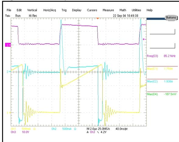
Figure 27. Steady State Vin=850V Pout=150W
