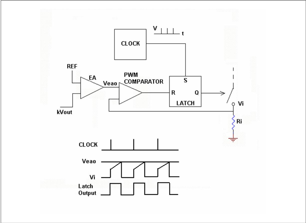
Figure 17. Implementation of Slope Compensation
