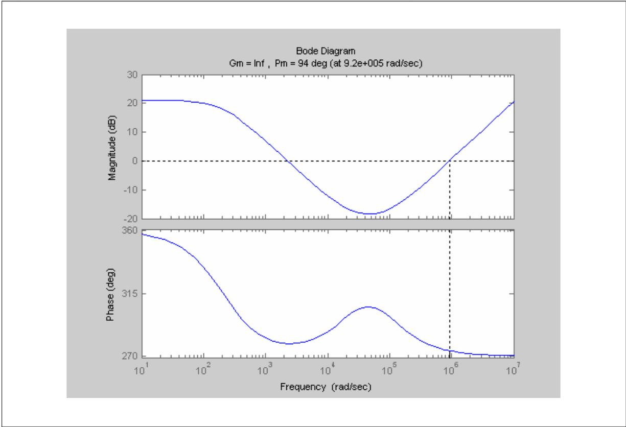
A good line and load regulation implies a high DC gain, thus the open loop gain should have a pole at the origin. Normally, in this case we need a feedback network like the one in figure 7. Its transfer function is given by:
