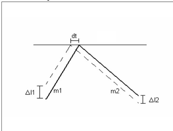
**Figure 15. Current Disturbance Effects at Duty Cycle >50%**
