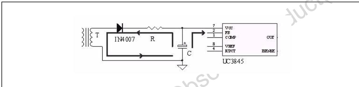
2. The auxiliary winding should be twisted tightly on the outermost layer and concentrated on the middle of the bobbin.
