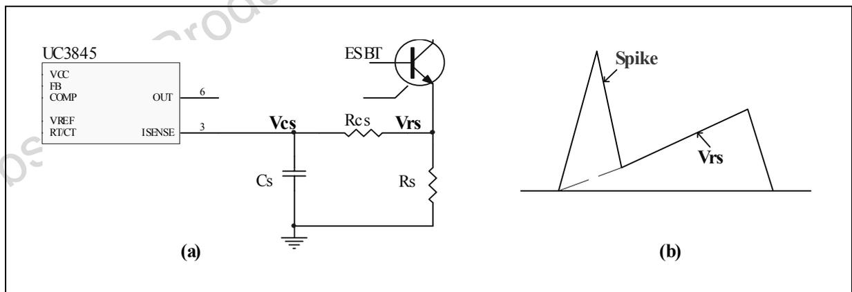
Figure 10: Normal Operation Waveforms of Output Pulse and Current Spike
