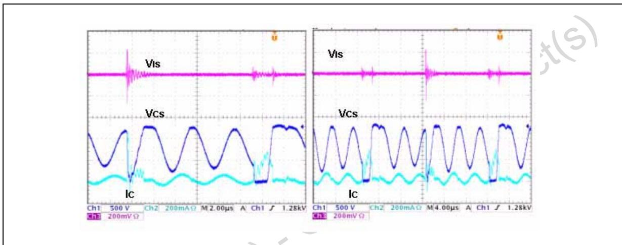
Note that in Figure 16 the oscillations are slightly decreased at min load and max input voltage when the heat-sink is not grounded (lower parasitic capacitance).
