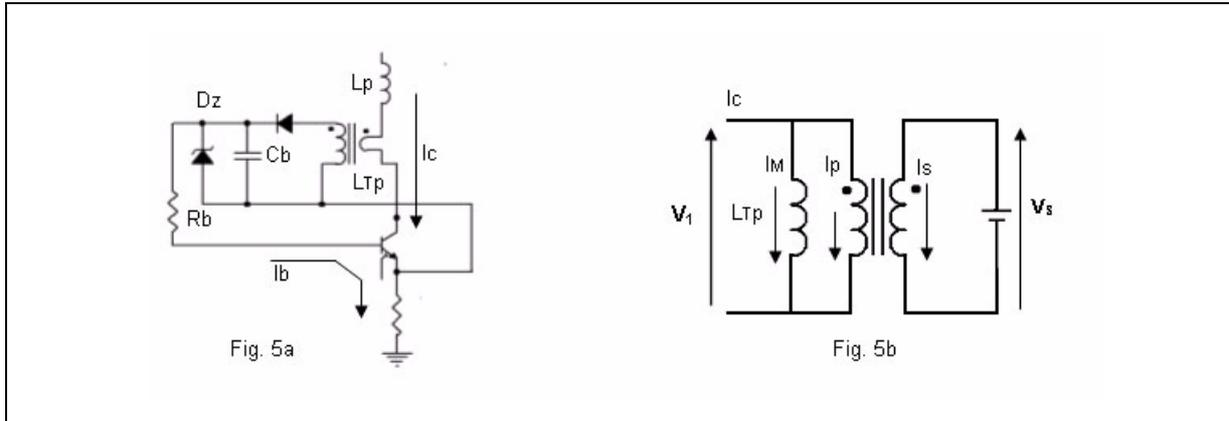
The current transformer turn ratio imposes a zone in the current characteristics with fixed  $I_C/I_B$ , its turn ratio has to be designed according to the characteristics of the chosen transistors and in particular to its gain. As an example, the STC03DE170 exhibits  $h_{fe}=5$  at  $I_C=1.8A$ ,  $V_{CE}=5V$ , so that in order to ensure the right saturation level of the transistor at full load operations we can fix at first a turn ratio:
