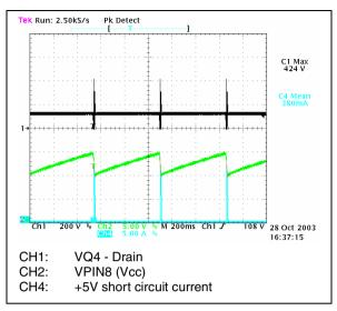
Figure 18. Short circuit on 5V @265 V<sub>AC</sub> - 50Hz - full load
