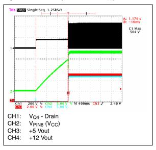
Figure 15. Start-Up Behaviours @full load - @90 V<sub>AC</sub> - 60Hz
