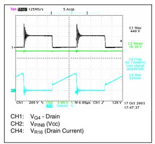
Figure 3. Drain voltage & current @230 V<sub>AC</sub> - 50Hz - full load
