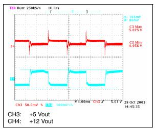
In Figure 13 it is reported the response of the output voltages for a load variation of the 12V output as detailed on top of the picture. The measurement has been done varying the 12V load from 50% to 100% load: the voltage variation is around 340mV and the 5V output is almost unaffected. Therefore, the conclusion is that there is no abnormal behaviour of the SMPS generated by a load change, allowing a good confidence for the integration of the SMPS in the equipment.
