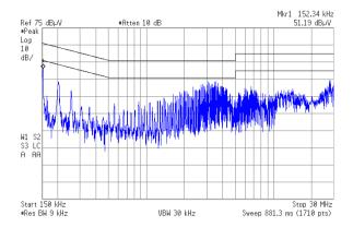
Figure 25. EN55022 Class-B Peak Measure 230 V<sub>AC</sub> - 50Hz - FULL LOAD
