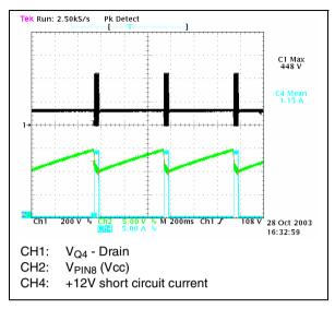
Figure 20. Short circuit on 12V @265 V<sub>AC</sub> - 50Hz - full load
