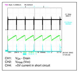
Figure 23. Short circuit on 12V @265 V<sub>AC</sub> - 50Hz - standby load
