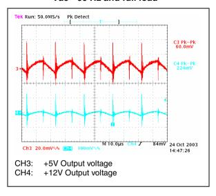
In figure 11 the output voltage ripples at switching frequency are measured. As shown, the ripple and the spikes are very low thanks to the additional LC filters added on both output and avoiding the use of bigger or expensive output capacitors.
