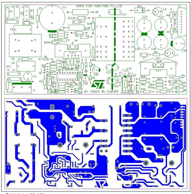
■ Original size: 89x180mm■ Copper thickness: 70µm
