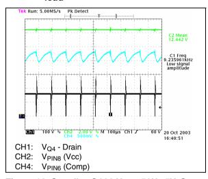
Figure 10. Standby @230 V<sub>AC</sub> - 50Hz 5V @ 50mA load
