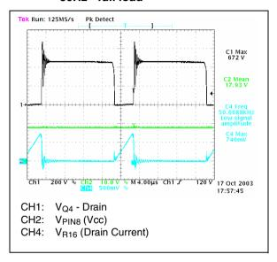
Figure 5. Maximum rectifiers PIV @Vin = 265 V<sub>AC</sub> - 50 Hz and full load
