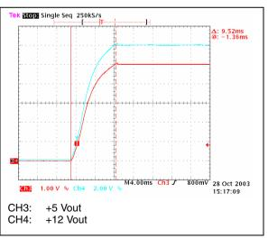
In the above picture the rising slopes at full load of the output voltages at minimum input mains voltage are captured and the rise time is measured. As shown in the pictures, the rising time is monotonic and it is almost constant overall the input mains range. No any overshoot or abnormal behaviour is present overall the input main range.
