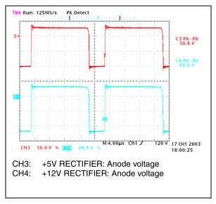
Here following the most salient controller IC signals are shown. In both pictures it is possible to distinguish clean waveforms free of hard spikes or noise that could affect the controller correct operation.
