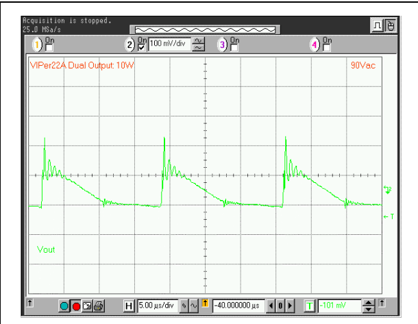
Figure 12. Switching ripple for 12V output
