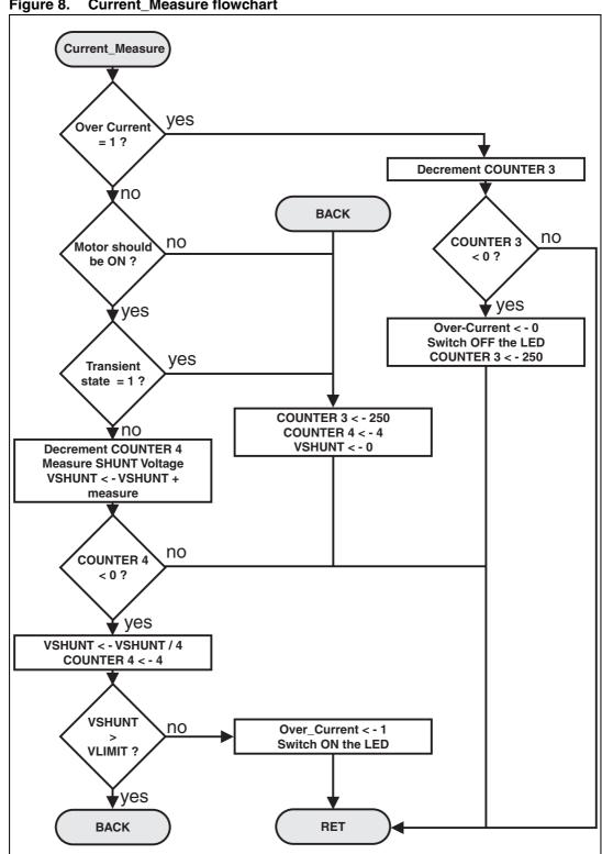
Figure 8. Current\_Measure flowchart
