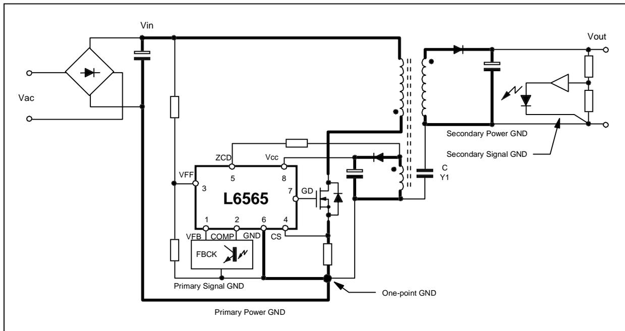
**Pin 7 (GD).** Gate driver output. It is able to drive an external MOSFET with 400mA source and sink capability. The driver is made up of a totem pole with a low side NDMOS. Its inherent body diode avoids the use of an external diode to prevent excessive negative voltages on the pin due to parasitic ringing.
