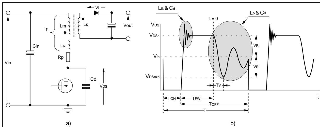
$C_d$  is the total capacitance of the drain node. It is the sum of the MOSFET's  $C_{OSS}$ , transformer intrawinding capacitance, stray capacitance due to the layout of the circuit (e.g. a heatsink) as well as other contributions reflected from the secondary side, such as an R-C damper on the rectifier diode.
