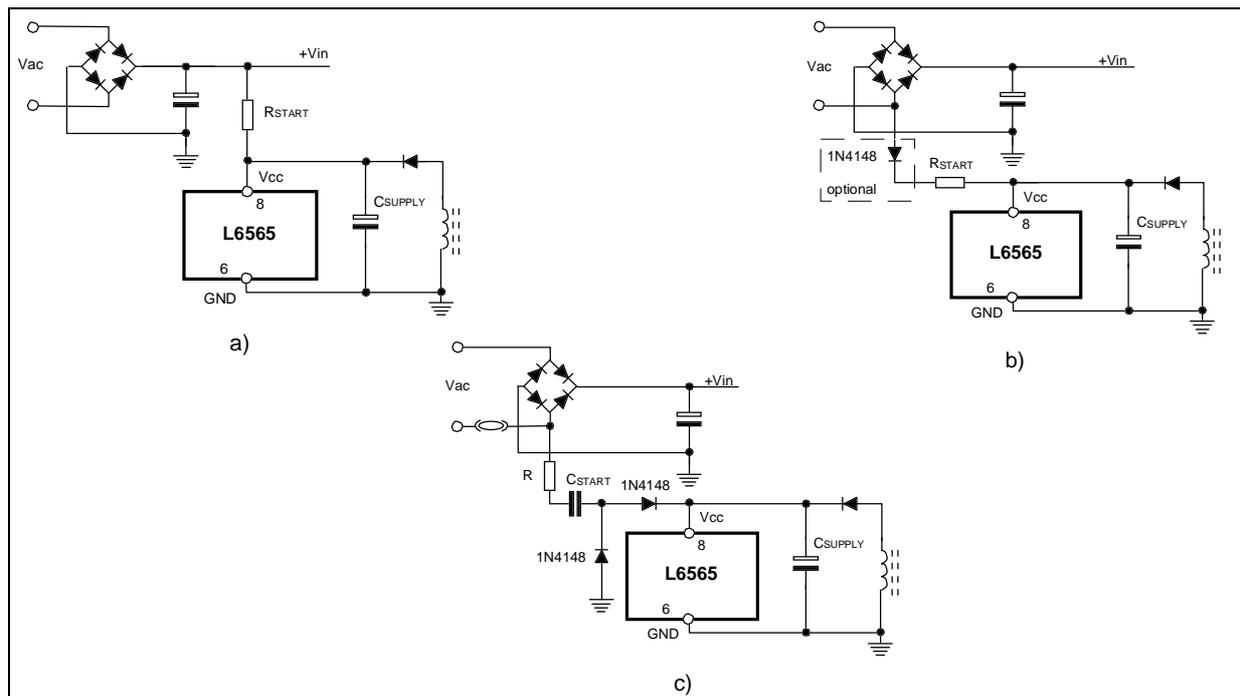
An additional film capacitor (0.1 or 0.22  $\mu\text{F}$  typically), placed as close the IC's pins as possible, can be used for filtering out the noise due to layout issues.
