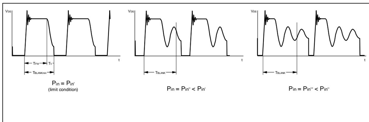
If the load current and the input voltage are such that the condition (22) is not fulfilled, the system will enter the "Frequency Foldback" mode, a sort of "ringing cycle skipping" illustrated schematically in figure 10.
