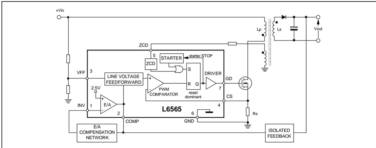
The total conversion cycle period  $T_{SW}$  is the sum of  $T_{ON}$ ,  $T_{FW}$  and  $T_v$ , and the switching frequency is:
