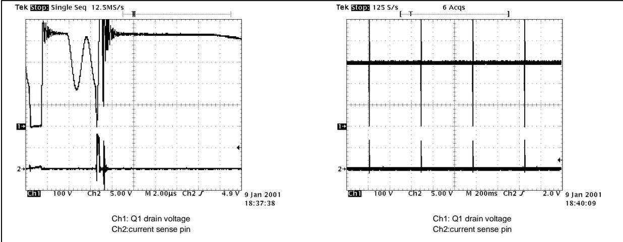
Figure 29. Uneven ringing cycle skipping during frequency foldback
