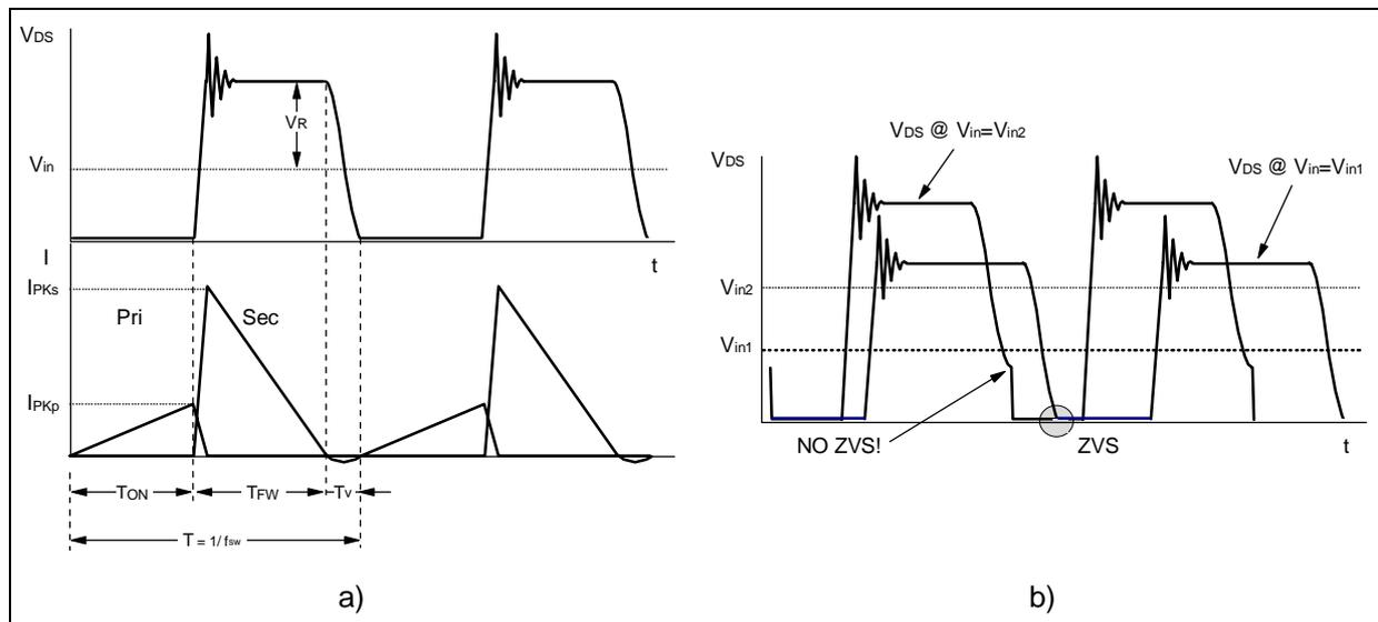
It is worthwhile noticing that the operation of the tank circuit depends only on circuit parameters and not on the operating conditions of the converter. The input voltage just impacts on the zero-voltage condition, as stated by eqn. 5 and shown in figure 2b.
