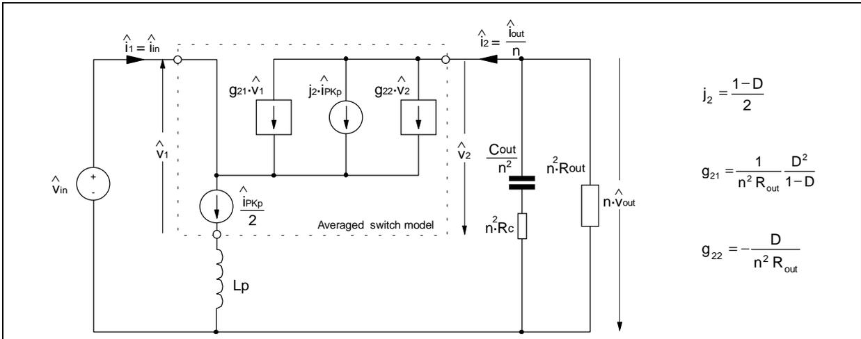
$$G2'(j\omega) = \frac{\hat{V}_{out}}{\hat{I}_{PKp}} = \frac{n R_{out} (1-D)}{2(1+D)} \frac{(1 + j\omega R_c C_{out}) \left( 1 - j\omega \frac{L_p}{n^2 R_{out} (1-D)^2} \right)}{1 + j\omega \frac{R_{out} C_{out}}{1+D}}$$
