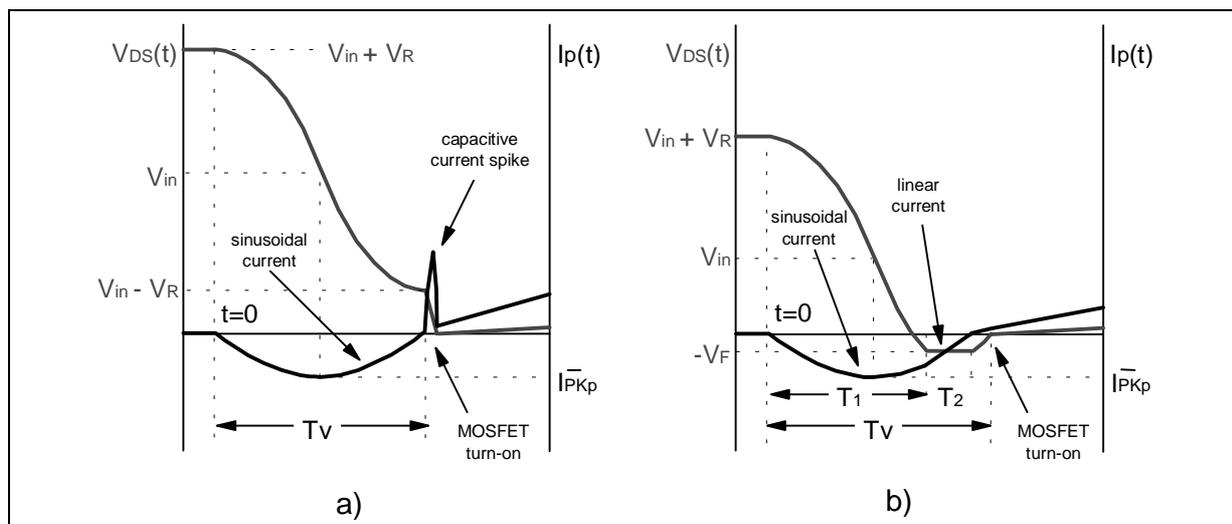
This being a reactive current, the associated power dissipation inside the MOSFET is ideally zero, negligible in practice. Some power is dissipated in the equivalent resistance of the primary winding, like in a standard flyback converter operated in DCM.
