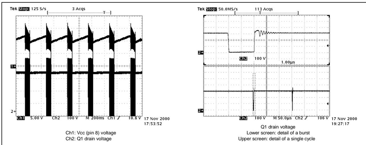
Figure 28. Short circuit of the output diode D5: detail of turn-on (left), Hiccup-mode operation (right).
