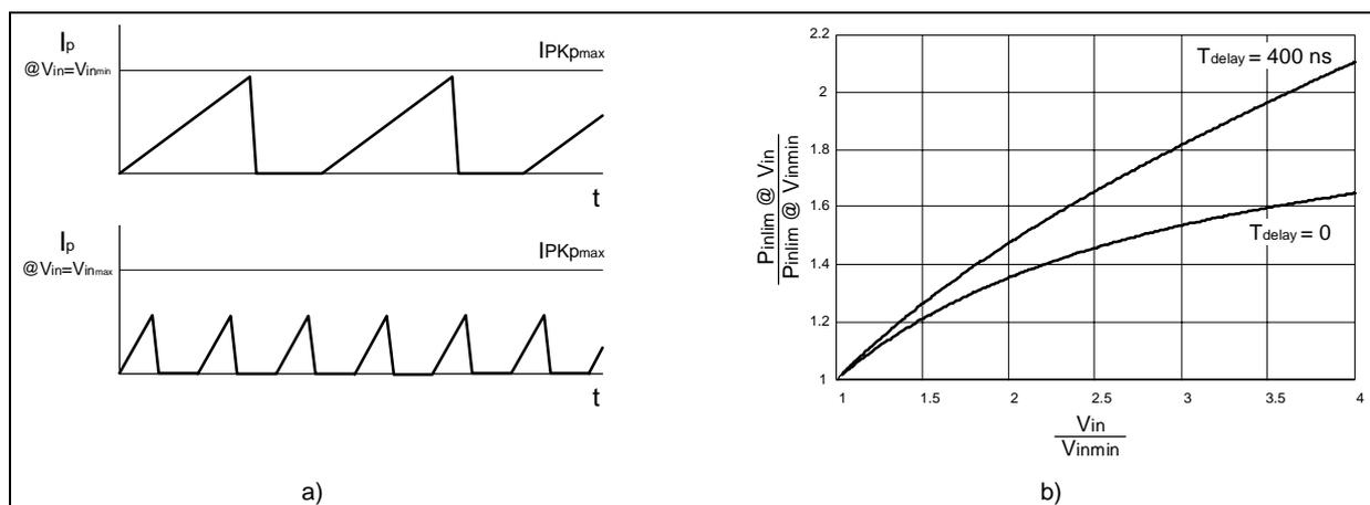
The effect of such delay is shown in figure 6b, where  $P_{inlim}$  vs.  $V_{in}$  is shown for both zero and 400 ns delay in a typical design ( $V_{in} = 100$  to  $400V$ ;  $P_{inlim} = 125W$ ,  $f_{swmin} = 100$  kHz,  $L_p = 110\mu H$ ,  $V_R = 150V$ ,  $C_d = 1.5nF$ ).
