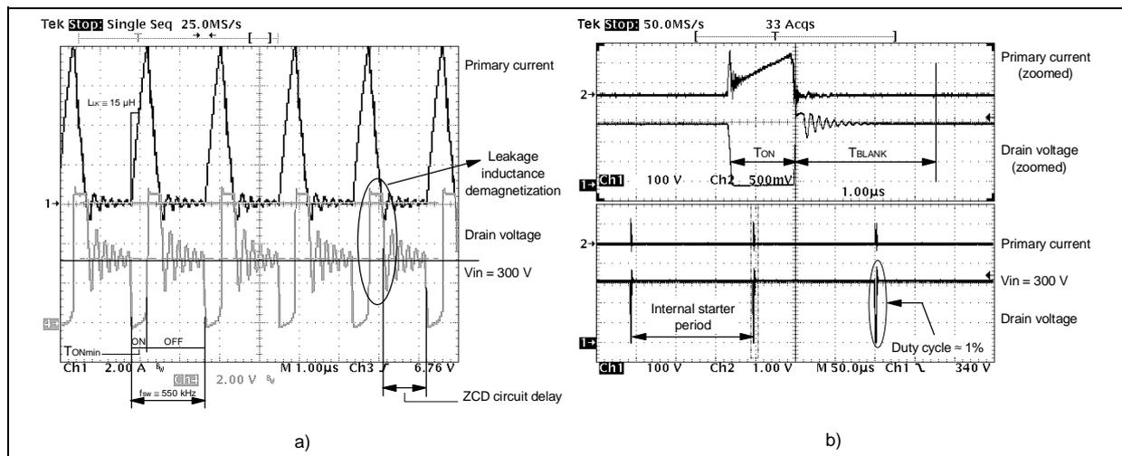
Figure 9b shows instead the operation previously described, allowed by the L6565, where the converter works at the frequency of the internal starter with a duty cycle of about 1%.
