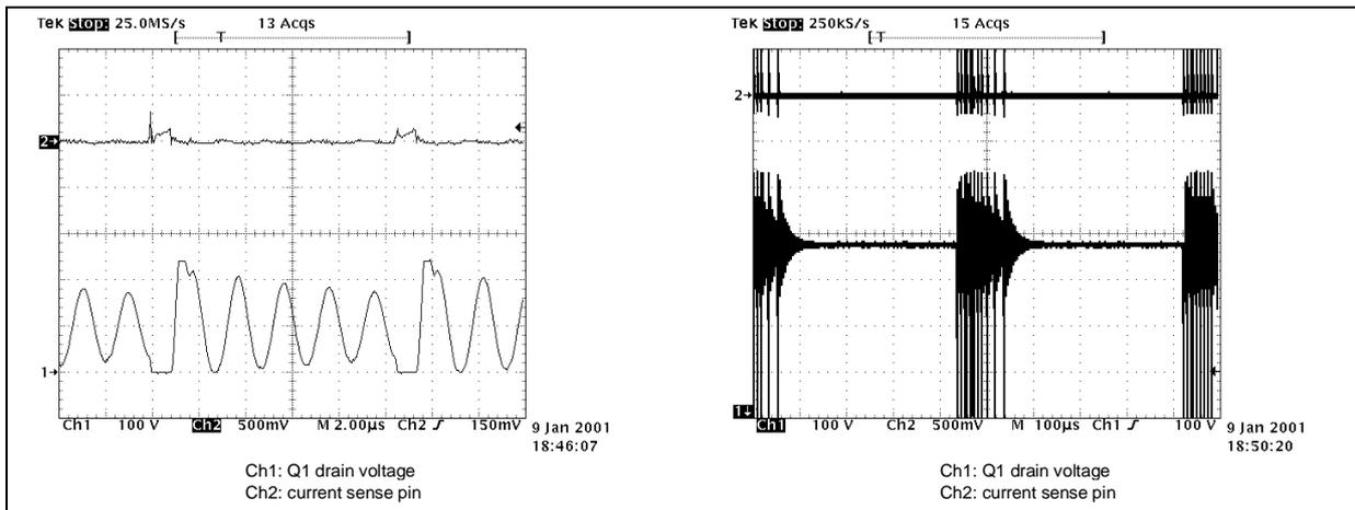
**Figure 27. Short circuit on 105V output,  $V_{in} = 300\text{ Vdc}$ : system running at the starter frequency**
