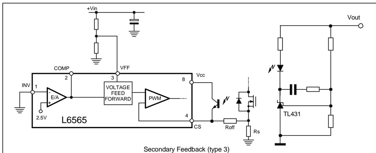
The E/A of the L6565 is not used at all for regulation and stays unbalanced high. This feedback arrangement is recommended when the device is required to work in synchronized mode and not as a QR controller. In fact, being the E/A output saturated high, the blanking time of the ZCD is fixed at  $T_{BLANKmin} = 3.5 \mu\text{s}$ , thus allowing the IC to be synchronized up to frequencies over 250 kHz, regardless of the line/load conditions.
