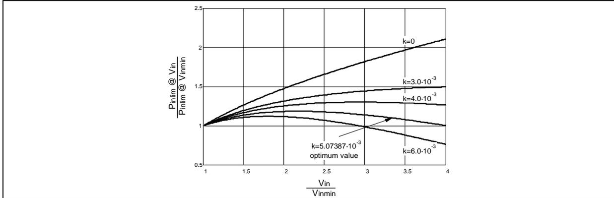
The diagram of figure 6b, as well as equations 14 and 15, shows a non-linear relationship between  $P_{inlim}$ ,  $V_{in}$  and  $V_{CSX}$ , hence the linear correction (17) will not result in a perfect compensation. A considerable reduction of the power capability change over the input voltage range will be achieved anyway.
