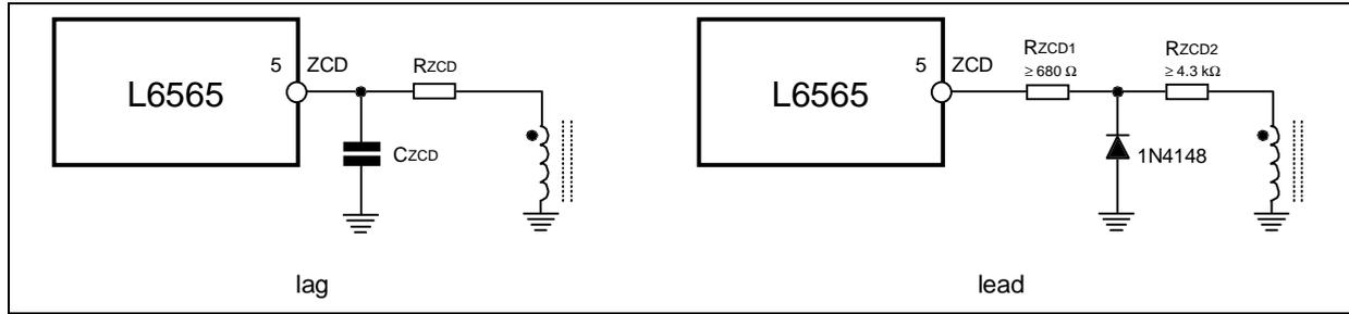
If the pin is driven by an external signal, the L6565 will be synchronized to (the negative-going edges of) that signal. To work properly, its period must be greater than the ZCD blanking time, its high level  $V_{s\max}$  greater than 2.1V and its low level  $V_{s\min}$  lower than 1.6V.
