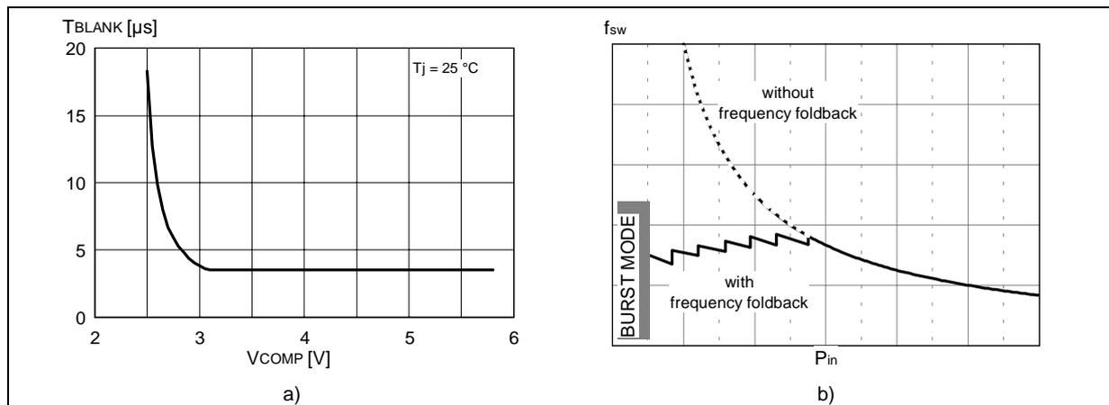
Any negative-going edge of the voltage at pin 5 that occurs during the blanking time is ignored; the first negative-going edge after  $T_{BLANK}$  has elapsed will trigger the ZCD circuit and determine MOSFET's turn-on.
