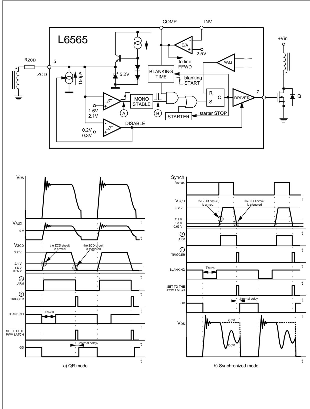
Figure 17. Frequency Foldback: timing diagram showing ZCD operation at light load
