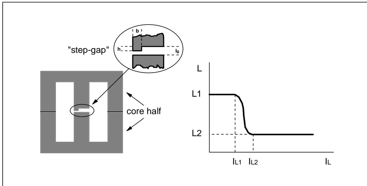
The appropriate height  $h$  and breadth  $b$  of the ferrite step (both of them determine  $L_1$  and  $I_{L1}$ ) for a given application will be found empirically.
