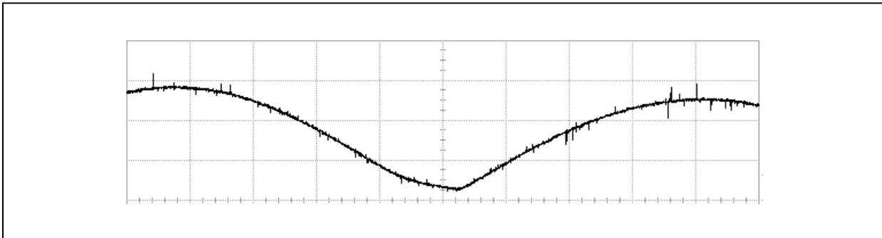
The obvious way of improving this is to lower the high frequency capacitor value. Care must be taken not to lower the capacitance such that the effectiveness of the EMI filter (in front of the diode bridge) is not degraded so as to not pass regulatory requirements. So, by lowering that capacitance, the HF filter capacitor in front of the diode bridge may need to be increased.
