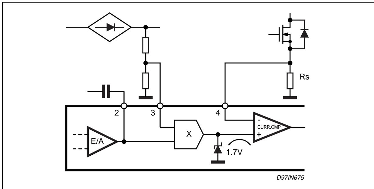
*Zero crossing dead time.* Once the multiplier operating parameters have been met, the input voltage as well as the input current should be looked at together. One problem to look for is a distortion of the current waveform especially at high line and low load. An example can be seen in figure 3.
