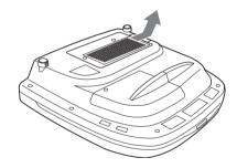
**4** Remove the air filter from the 6 tabs of the air filter cover.
