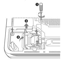
**5** While holding the handle and keeping the lamp unit horizontal, pull straight up.
