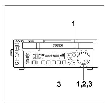
In shuttle mode, the SHUTTLE dial controls the playback speed based on the angular position of the dial. There are seven playback speeds:  $\pm 0.03$  times,  $\pm 0.12$  times,  $\pm 0.5$  times,  $\pm 1$  times,  $\pm 2$  times,  $\pm 1$  times,
