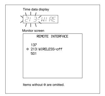
**2** Turn the JOG/SHUTTLE dial to change the setting from "OFF" to "ON" while holding down the JOG/SHUTTLE button, and then release the JOG/SHUTTLE button.
