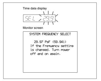
4 Holding down the JOG/SHUTTLE button, turn the JOG/SHUTTLE dial to change the setting to 25, then release the JOG/SHUTTLE button.
