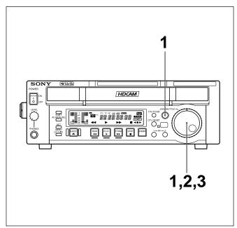
In jog mode, the JOG dial controls the playback speed based the speed at which the dial is turned. The playback speed range is  $\pm 1$  times normal speed. Use the following procedure to carry out playback in shuttle mode.
