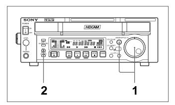
1 Holding down the JOG/SHUTTLE button, turn the JOG/SHUTTLE dial.
