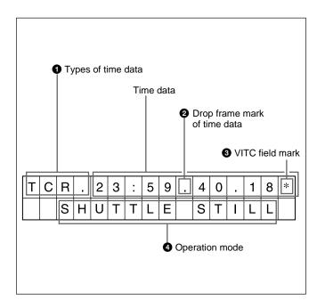
Video signal output from the SDI (J-H3 only), HD SDI (J-H3 only), COMPOSITE, COMPONENT (Y/Pb/Pr), D3 or MONITOR connectors contains superimposed character information (overlaid display), including time code, menu settings, or alarm messages.
