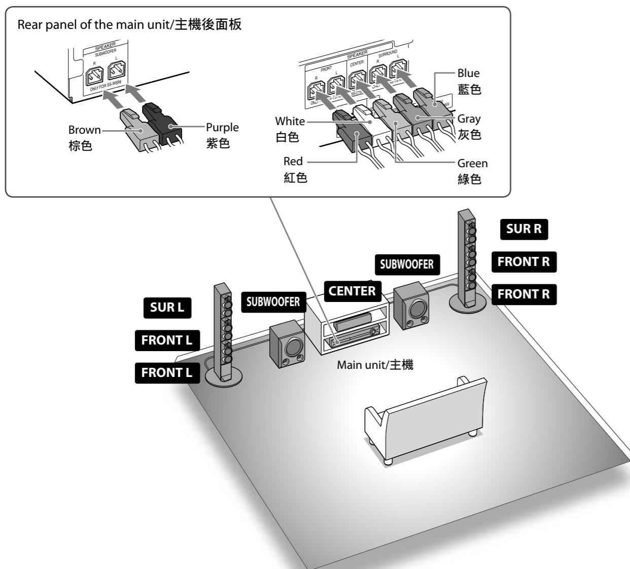
**To connect speaker cords to the center speaker and subwoofers/將揚聲器導線連接到中置揚聲器和低音揚聲器**
