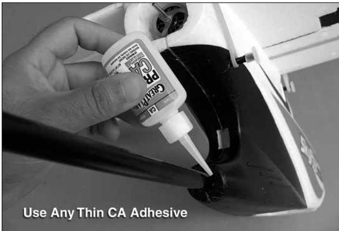
❑ 4. Being careful not to disturb the alignment, wick about 5-8 drops of regular thin CA into the tail boom to fuselage pod joint. Carefully set the model aside and let the glue dry. **Note:** If you ever need to debond the CA joints, please purchase Great Planes CA debonder (GPMR6039).
