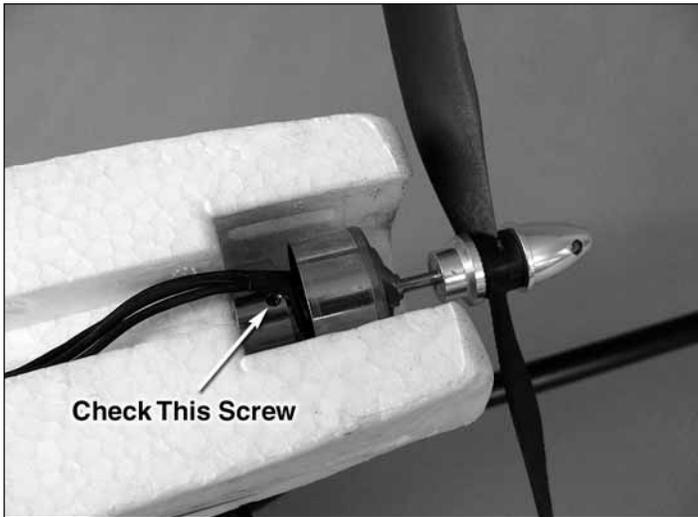
From time to time, check the motor to make sure that vibration has not loosened it on the mount. Tighten the motor mount set screw if it has loosened.
