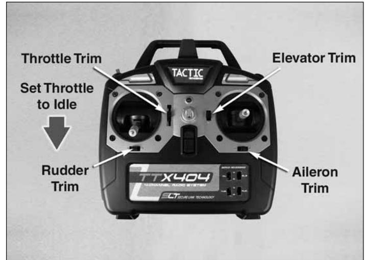
❑ 7. Set the throttle stick (left stick) to idle (all the way down) and turn on the transmitter. The power indicator light should be glowing a steady red. A flashing red light indicates low voltage. If this is the case, replace the batteries before connecting your flight battery pack.
