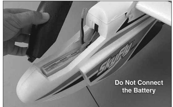
❑ 6. Set the battery in the battery compartment, but do not connect it. Fit the canopy. You will need all these in place when you balance the model.
