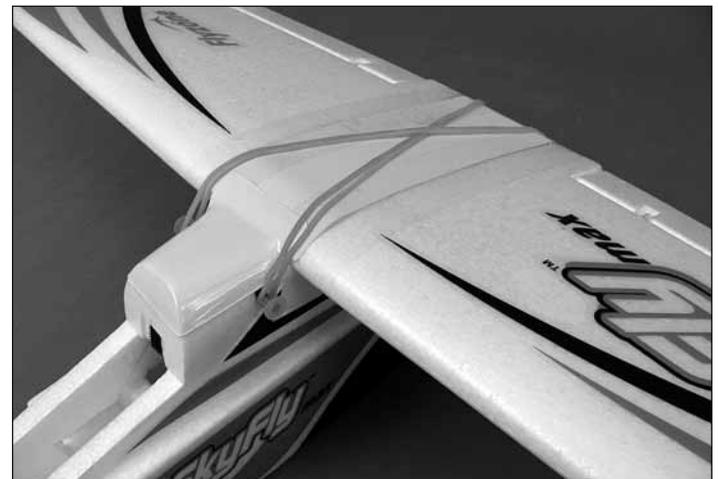
❑ 1. Temporarily fit the wing to the fuselage using two of the supplied 8" [203mm] rubber bands.
