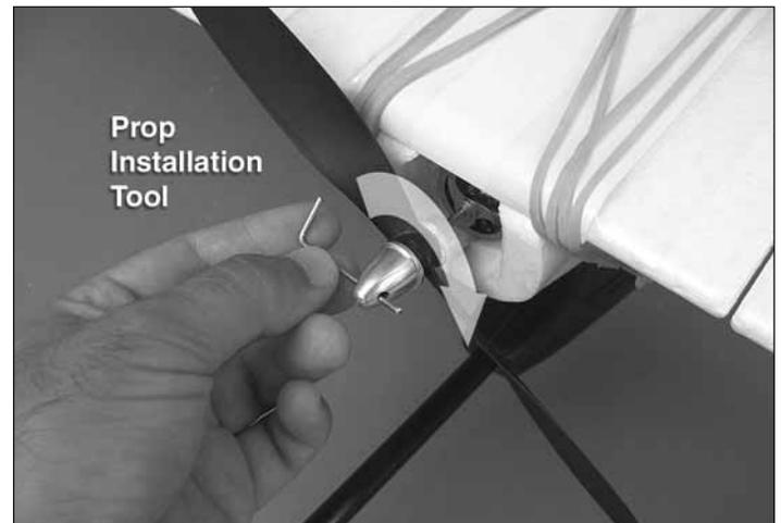
❑ 7. Install the propeller to the motor shaft. Use the prop installation tool to tighten the spinner nut.
