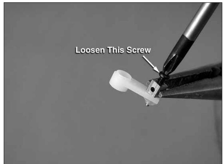
❑ 13. Carefully unscrew the pushrod locking screw from the screw-lock pushrod connector. You do not need to completely remove the screw – loosen it until you can slide the pushrod freely through the hole. **Note:** The screw threads are coated with thread locking compound, so you will need to grip the body of the screw-lock pushrod connector with a pair of needle-nosed pliers.
