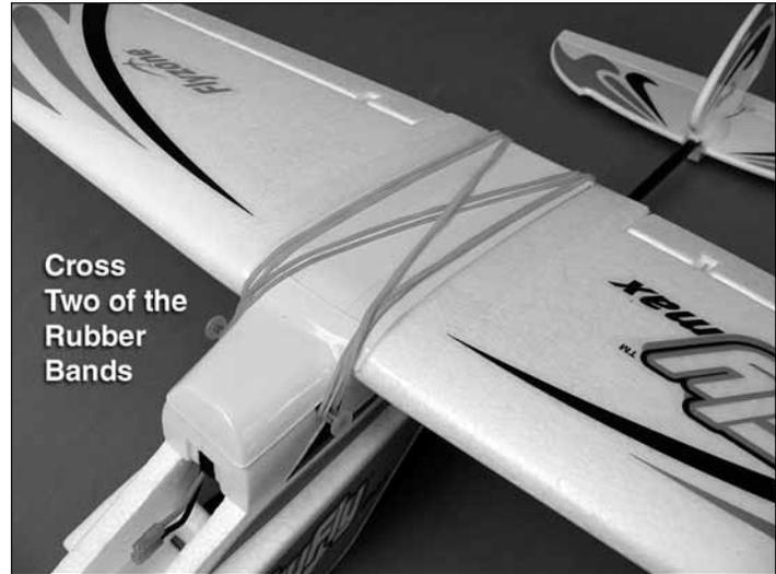
☐ 1. Tuck the wires into the fuselage and fit the wing. Install the wing using the four supplied 8" [203mm] rubber bands. Cross one pair as shown. Make sure that the wing is sitting correctly and that the servo wires are not caught between the wing saddle and the wing.
