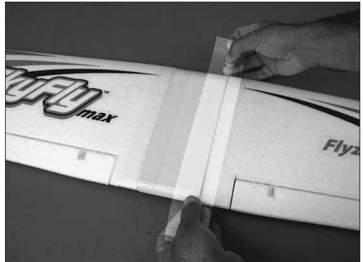
❑ 3. Turn the wing over. Peel the backing paper off of the supplied 11-3/4" [300mm] piece of wing joining tape. Apply the tape so that it secures the plastic center wing piece to the right wing. Wrap the tape around the wing and trim off any excess tape with scissors.
