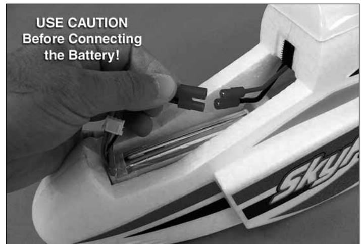
❑ 10. Steps 10 through 22 require you to power the radio system. With the transmitter still on, plug the LiPo battery into the speed control (ESC) connector. When the
