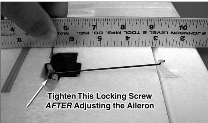
☐ ☐ 22. Loosen the aileron pushrod locking screws. Use a straight edge to set each aileron to zero travel (centered). With the aileron set, tighten the pushrod locking screw. Check to see that the aileron stayed centered and that the linkage is secure.
