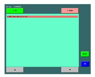
(3) Touch the **[PRINT]** key, if the printout is required. Touch the **[OK]** key to close the guidance for the recipe.
