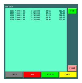
To operate the reorder entries, touch a corresponding line of the GLU list and touch the **[ENTER]** key. To exit from the GLU list screen, touch the **[CANCEL]** key.
