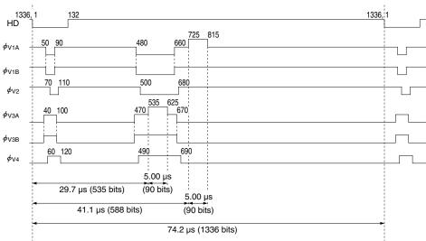
READOUT TIMING FOR 18.0 MHz OPERATION [FIELD ACCUMULATION MODE]
