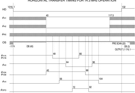
HORIZONTAL TRANSFER TIMING FOR 14.3 MHz OPERATION
