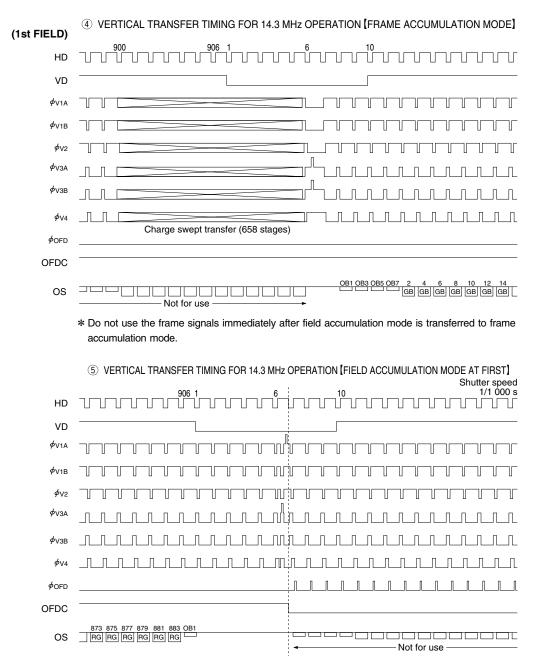
\* Do not use the field signals immediately after frame accumulation mode is transferred to field accumulation mode.
