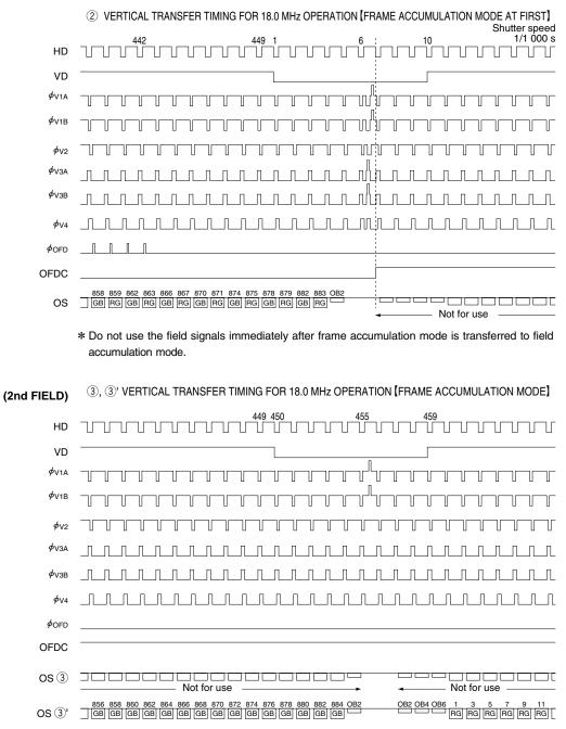
\* Do not use the field signals immediately after frame accumulation mode is transferred to field accumulation mode.
