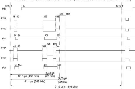
READOUT TIMING FOR 14.3 MHz OPERATION [FRAME ACCUMULATION MODE AT FIRST]
