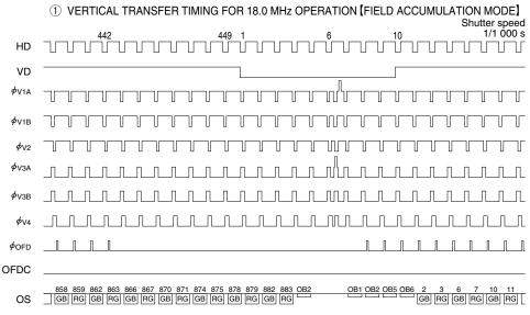
\* Do not use the field signals immediately after frame accumulation mode is transferred to field accumulation mode.
