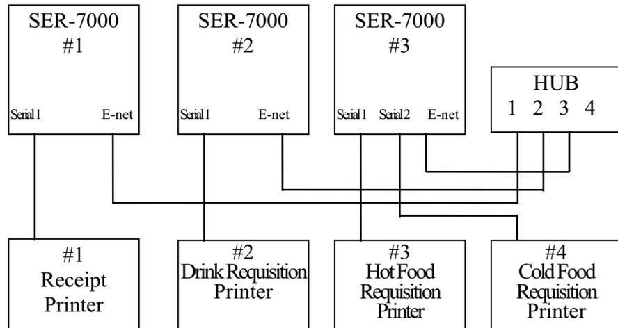
Within this system, printing instructions from any of the registers can be directed to the appropriate printer, for example:
