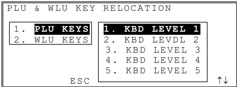
3. A pop up window displays the keyboard level selection. Select the keyboard level you wish to program, press **ENTER**.
