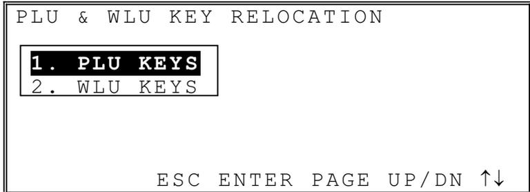
2. Press a numeric digit (1-2) or use the ↑ or ↓ keys to move the cursor to PLU KEYS or WLU KEYS, then press **ENTER** to indicate whether you wish to program a PLU or WLU.
