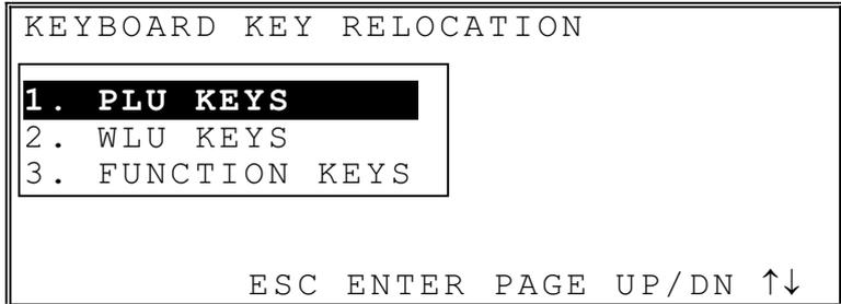
2. Press a numeric digit (1-3) or press the ↑ or ↓ keys to move the cursor to your choice. Then press **ENTER** to indicate whether you wish to program a PLU, WLU or FUNCTION key.
