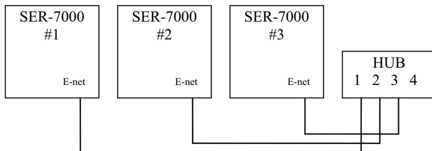
Contact your SAM4S sales representative to order the appropriate Ethernet hubs. Hubs will be stocked in 5 port and 8 port configurations.
