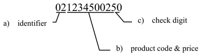
There are 11 identifier numbers available for non-PLU code programming: “02” and “20” through “29”. The purpose of this program is to define the format of the 10-digit part b for each possible identifier. For example:
