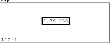
2. Enter the tare # and press the **SCALE** key to display the weight less the tare.
