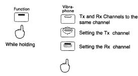
With the FUNCTION button still depressed, press the key which corresponds to the desired MIDI channel. (See illustration below.)
