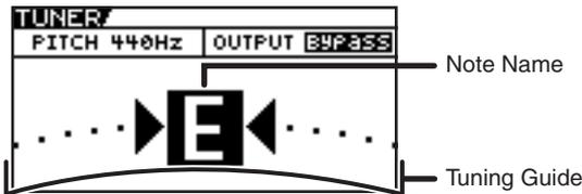
When the difference from the correct pitch falls within 50 cents, the Tuning Guide then indicates the size of that difference. As you watch the Tuning Guide, tuning until the center indicator lights up.
