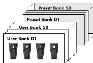
Patches include User patches, which you can use to save the settings for newly created effects, and Preset patches, for which modified settings cannot be saved. For more information, refer to "Selecting a Tone (Patch Change)" (p. 30).
