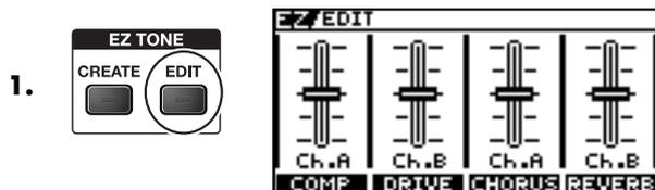
2. P1 knob: Adjusts the volume level of the compressor.
