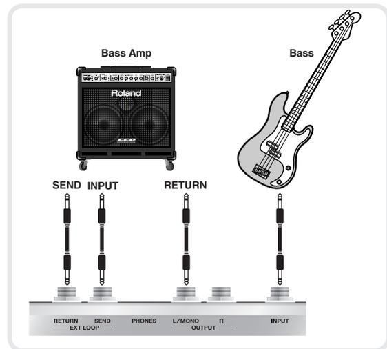
\* When you're making connections using the SEND/RETURN jacks, you also need to make settings for the "SEND/RETURN" (p. 131).
