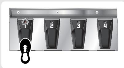
The indicator for the number pedal you pressed lights up and the patch is switched.
