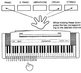
\* Each time power is turned on, the unit defaults to "1" as the channel used for both transmission and reception.
