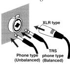
Both balanced and unbalanced connections are possible.
