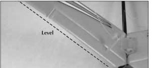
□ 5. Using the **adjustment knobs** on the **control horns**, adjust each control line until the elevon surfaces are level with V-tail fins.
