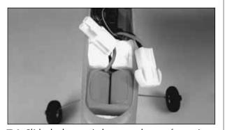
□ 2. Slide the battery in between the two foam pieces inside the fuselage with the connector facing the back of the plane. Push the battery until it is seated against the bottom of the fuselage. Do not connect the battery until you are ready to fly.
