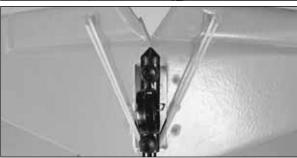
□ 4. Locate a small rubber band included with the Red Hawk. Hook the rubber band to the left **elevon control hook**. Loop the rubber band around the front of the V-tail tray and connect the rubber band to the right control hook.
