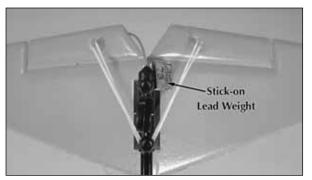
□ 3. If the model balances with your fingertips **ahead** of the lines, weight will have to be added to the **tail** to get it to balance. Tail weight may be stuck to the bottom of the V-tail at the center. Be sure that any added weight does not interfere with the operation of the elevons.
