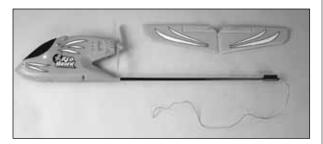
□ 1. Remove the **fuselage** from the packaging. Be careful when removing the fuselage from the packaging as the **control wire** that is preinstalled in the fuselage is connected to the **V-tail**. Lay the parts out on a table ensuring the control wires are not intertwined or twisted together. Until the red antenna wire and let it hang freely. **Do not cut off excess antenna wire!**
