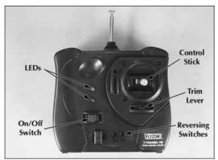
When the control stick is moved **down**, the elevons will move **up** together. When the control stick is moved **up**, the elevons will move **down** together. When the control stick is moved **right**, the left elevon will move **up** and the right elevon will move **down**. When the control stick is moved **left**, the left elevon will move **down** and the right elevon will move **up**.
