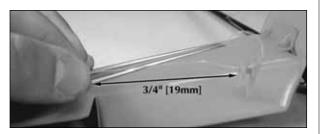
□ 7. Feed the wire through the hole in the control horn and then through the hole in the adjustment knob. Pull approximately 3/4" [19mm] of excess wire through the knob.
