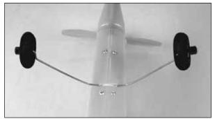
□ 1. Locate the **main landing gear**. Squeeze the wheels together as shown in the picture and push the center of the landing gear wire into the slot as far as it will go into the underside of the fuselage body. Let go of the wheels and they will spring back into position securing the gear to the plane.
