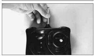
☐ 1. Locate the antenna and screw it into the top of the transmitter.
