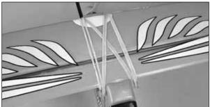
□ 1. Center the **wing** onto the fuselage. Use the alignment bump at the front of the wing by positioning the wing so the bump is even with the mold line in the fuselage body. Secure the wing to the fuselage using four of the included **large** rubber bands. Hook the rubber bands onto the front and rear **rubber band pegs**. Attach two rubber bands straight and two diagonally as shown in the picture.
