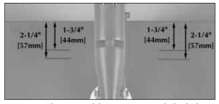
□ 1. Use a fine-point felt-tip pen to mark the balance range on both sides of the bottom of the wing according to the measurements shown in the photo. Note that the measurements are from the front, or leading edge of the wing.
