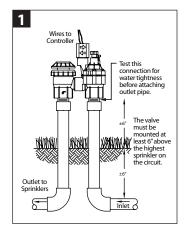
Do not connect the outlet side (piping to sprinkler heads) without first testing for leaks. If the outlet side is connected and there is a leak, the pipe would have to be cut in order to tighten the connection.
