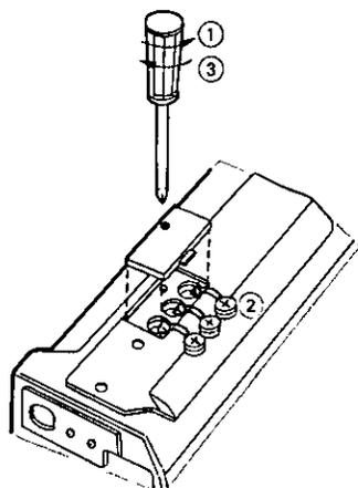
The VHS Movie has an auto date function which calculates the date and time, including leap year, automatically until Dec 31 1999. This function is activated by the battery even when the VHS Movie power is off. The battery must be inserted before date and time can be kept automatically as follows.
