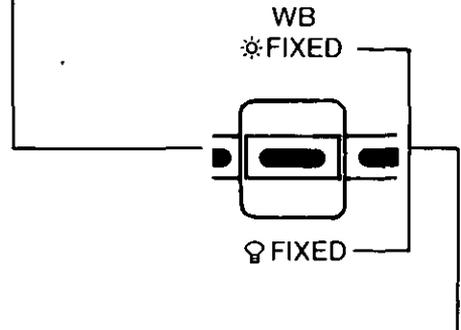
Under the following conditions it is recommended that you press and set the White Balance Switch to one of the FIXED positions for better color reproduction.
