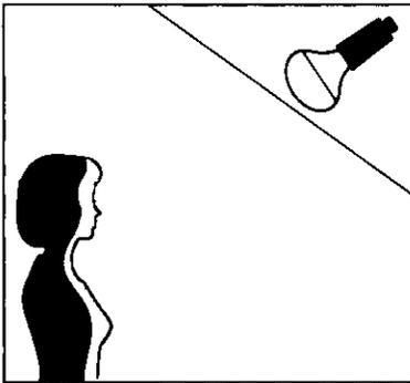
To prevent dark shadows when using a strong light, diffuse the light with tracing paper (but keep the paper far enough away to prevent a fire).
