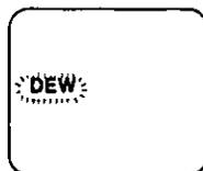
This indicator appears if excessive moisture condenses in the unit. If the DEW Indicator is ON, the unit will not operate. If this happens, the DEW Indicator will flash for about 10 seconds and the VHS Movie will automatically turn off. In this case, wait until the indicator no longer flashes when the VHS Movie is turned on again.
