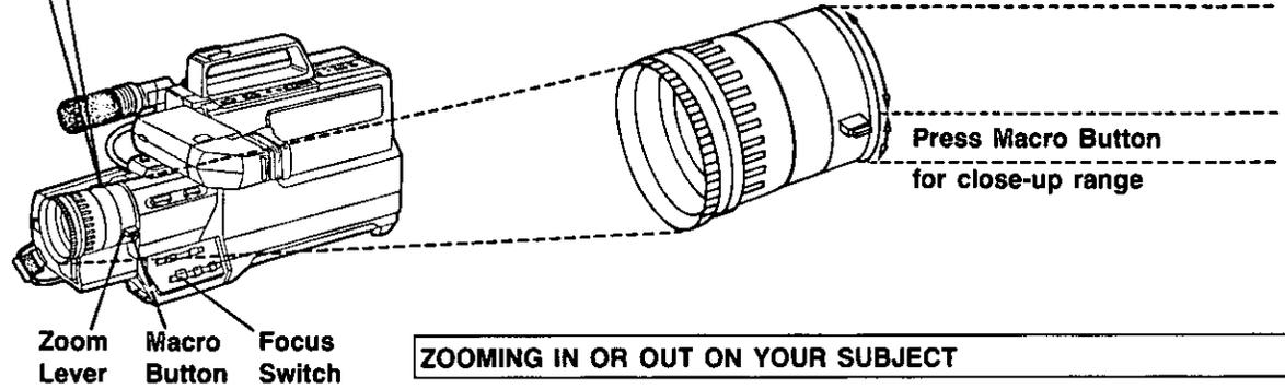
The VHS Movie has a power zoom lens that gently changes the viewing angle. Zooming is possible by lightly pressing the T or W side of the Power Zoom Switch. The power zoom is conveniently located at your finger tips on the hand grip so you can control it with one hand while focusing with your left. You can also manually zoom at anytime; the zoom ring has a handy lever for steady turning.
