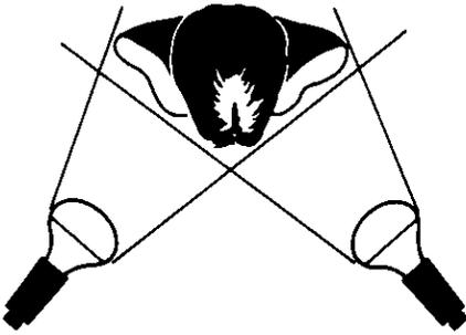
Lighting is often necessary to achieve sufficient brightness for a good picture. It is also an art in itself. Many amateurs simply mount a light on the VHS Movie or use two lights parallel to the VHS Movie on either side. This simple approach creates strange shadows and tends to make the subject look flat. (See diagram.)
