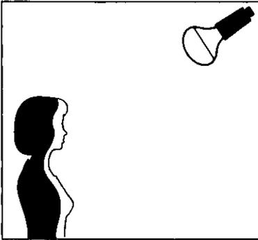
For a more three-dimensional effect, the main light should be raised so that it is at a 45° vertical angle.
