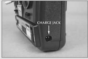
The Tactic 4-channel transmitter is equipped with a charge jack that will allow you to use a rechargeable NiCd battery pack and charge it directly through the transmitter. For a rechargeable pack that works with this transmitter, use part number FUTM1450 Transmitter NiCd 9.6V 500mAh.
