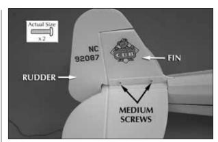
□ 4. Remove the two screws in the fin holder and insert the fin into the fin holder. Reinstall the two screws to secure the fin to the holder. Be careful to not overtighten the screws.
