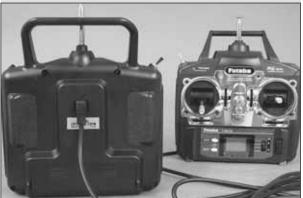
The Tactic™ transmitter is equipped with a trainer system that, when used with another Tactic or Futaba® transmitter, can transfer airplane control to a second pilot for learning purposes.
