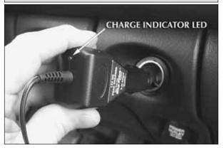
□ 1. Plug the battery charger into a 12-volt power outlet in a vehicle, placing the battery to be charged outside the car, and away from flammables. **NEVER** charge your airplane battery while driving or with the vehicle engine running!
