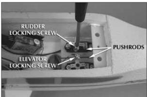
□ 5. With the transmitter and plane switched on, center the elevator, rudder and aileron sticks and trim levers. Use a straight edge to adjust the rudder and elevator so that they are in the neutral position and tighten the screws in the pushrod connectors.
