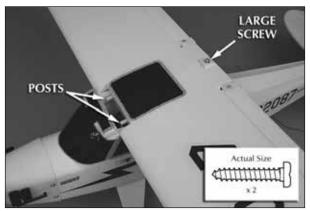
□ 2. At the front edge of the wing are two small posts. Position the wing on the top of the fuselage and slide
