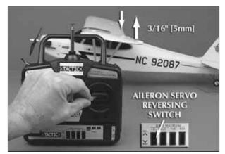
□ 3. By moving the right control stick left, the left aileron must move up and the right aileron must move down. If they do not, change the position of the aileron servo reversing switch on the transmitter. When the right stick is moved all the way to the left, the trailing edge of the left aileron at the inward side should move **up** 3/16" [5mm]. When the right side stick is moved all the way to the right, the left aileron should move **down** 3/16" [5mm].
