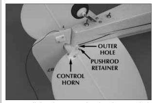
☐ 4. Install the elevator pushrod in the outer hole of the control horn. Slide a pushrod retainer over the pushrod to secure it.
