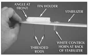
□ 2. Insert the two threaded rods of the fin holder through the stabilizer, making sure that the white control horn is on the bottom.
