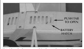
□1. After the battery pack is charged, open the battery hatch. Insert the battery pack inside the fuselage. Do not plug the battery pack into the connector inside the fuselage. Close the battery hatch.
