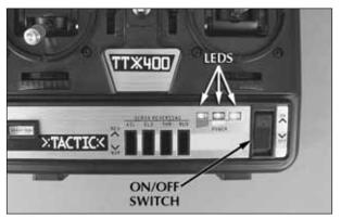
□ 5. Switch on the transmitter and check the LED on the front of the transmitter. The LEDs keep
