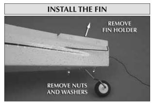
☐ 1. Remove the two nuts and washers on the bottom aft end of the fuselage. Then, remove the fin holder from the fuselage.
