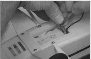
□ 1. Switch on the transmitter. Make sure all three LEDs are on. Open the battery hatch cover on the bottom of the plane and insert the battery. Attach the battery to the connector. Turn on the plane by moving the switch on the left side of the fuselage.
