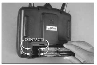
□ 4. Insert the battery holder in the transmitter case so that the two contacts on the battery holder align with the contacts in the transmitter case. Reinstall the battery hatch on the transmitter case.
