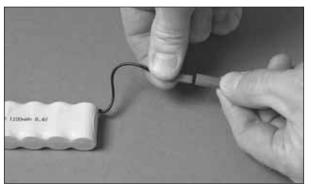
□ 2. Plug the battery pack into the charger connector. Be careful—do not force the plugs. The
