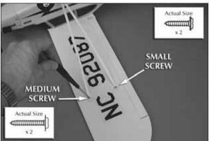
□ 3. Turn the plane over and attach the wing struts to the battery tray using two small screws. The arm of the wing strut that goes towards the front of the wing is marked with an arrow. Attach the other end of the wing struts to the wing using a small screw at the back edge of the wing and a medium screw at the front edge. Repeat this procedure forth e other wing. Important: The Piper J-3 Cub must never be flown without the wing struts attached. The wing struts help support the wing.
