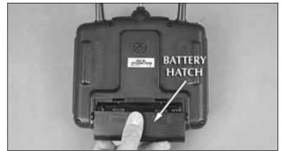
□ 2. The transmitter is the unit that controls your airplane and requires of eight good quality "AA" batteries. To install the batteries, remove the battery hatch on the back of the transmitter.
