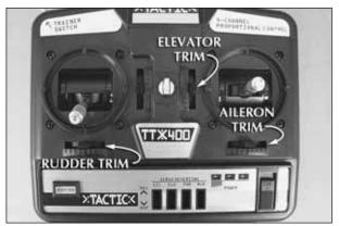
☐ 2. Center the rudder, aileron, and elevator trim.
