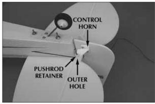
□ 3. Install the rudder pushrod in the outer hole of the control horn. Slide a pushrod retainer over the pushrods to secure it.
