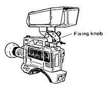
Note: When connecting the viewfinder cable of WV-VF65B to the viewfinder connector on the camera, use the viewfinder connector conversion cable (supplied) in between.
