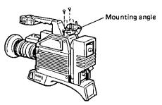
3. Attach the round viewfinder mounting base (supplied) to the mounting angle with two screws.
