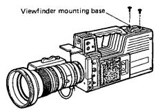
5. Slide the viewfinder adjusting angle into the mounting base and tighten the fixing knob to secure the viewfinder. Connect the viewfinder connector.
