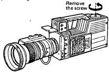
4. Attach the round viewfinder mounting base (supplied) to top of the camera with two screws.
