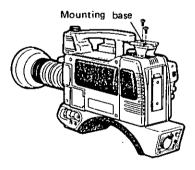
4. Slide the viewfinder adjusting angle into the mounting base and tighten the fixing knob to secure the viewfinder. Connect the viewfinder cable.
