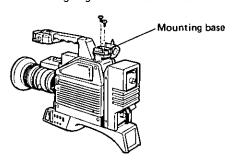
Slide the viewfinder adjusting angle into the mounting base and tighten the fixing knob to secure the viewfinder. Connect the viewfinder connector.
