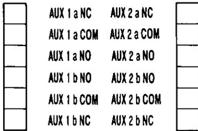
The AUX1 is composed of dual switching circuit such as AUX1 a, AUX1 b. (Same as AUX2)
