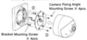
Mount the camera onto the Camera Mounting Angle.
