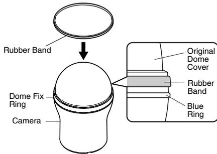
**2** After turning the dome fix ring to the left, remove the original Dome cover from the camera, and then remove the drip-proof packing.
