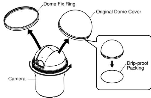
**3** Place the drip-proof packing removed in Step 2 onto the replacement Dome cover WV-CS3S, and put them on the camera.
