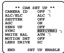
4. After confirming that the cursor is on EXT (VBS), press . The phase adjustment menu appears on the monitor.
