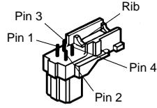
(2) Solder the lens cable to the pins of the supplied connector.
