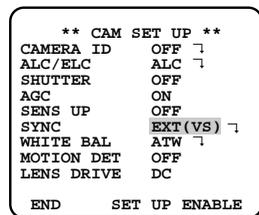
4. After confirming that the cursor is on EXT (VS), press . The phase adjustment menu appears on the monitor.
