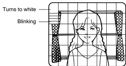
**Note:** If ON is selected for the SUPER-D2 parameter, a shadow (black line) may appear at the boundary between the bright and the dim scene. This is a natural phenomenon and does not indicate trouble.
