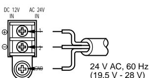
Recommended wire gauge sizes for 24 V AC line.
