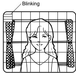
3. Move the cursor to the area where backlight is bright and press to mask that area. The mask turns to white. (When the cursor is moved on an area that has already been masked, the mask and cursor start blinking.)
