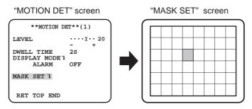
In the masked area, no alarm will be issued even if a moving object is detected. The masked area is set in the same way as the masked area setting in Light quantity control method selection. (Fig. page 11)
