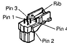
Solder the lens cable to the pins of the supplied connector.
