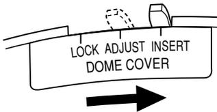
**Important:** For inner dome adjustments, adjust the marker to the position of "ADJUST". If the dome cover block is moved with unreasonable force, this may be a cause of destruction.
