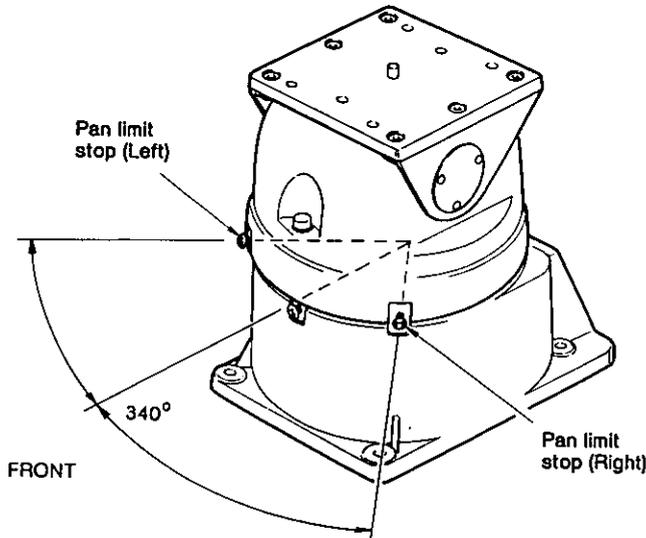
2. Turn on the ON/ OFF switch to energize unit, then rotate pan/tilt unit using joystick the pan/tilt control unit until desired right pan limit is reached.
