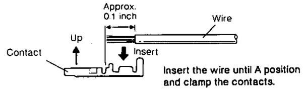
Prepare the individual conductors for clamping. If clamping, use MOLEX brand tool part number 57027-5000 (for UL-Style cable UL1015) or 57026-5000 (for UL-Style cable UL1007).
