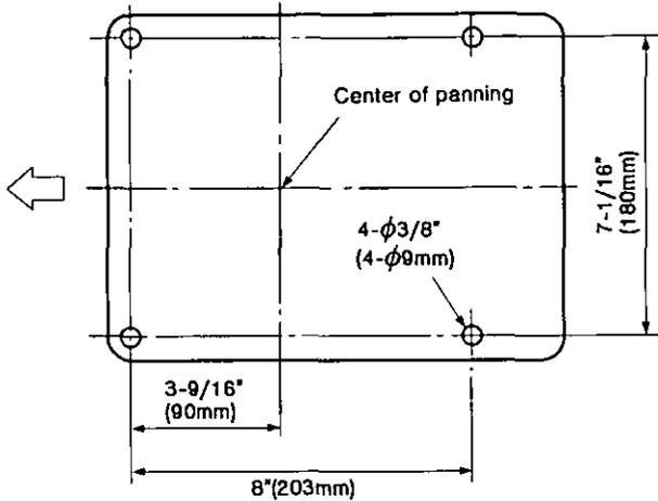
2. When mounting the outdoor camera housing on the Mounting Plate. Four M8x20 mm (5/16" x 13/16") hex head bolts, plain washers and lockwashers are provided with the Pan/Tilt Unit. Use these to mount the camera housing as shown below.
