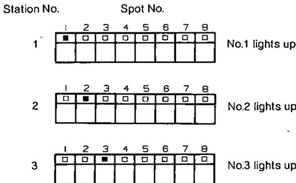
b. The Bypass LED shows the unit number as follows.
