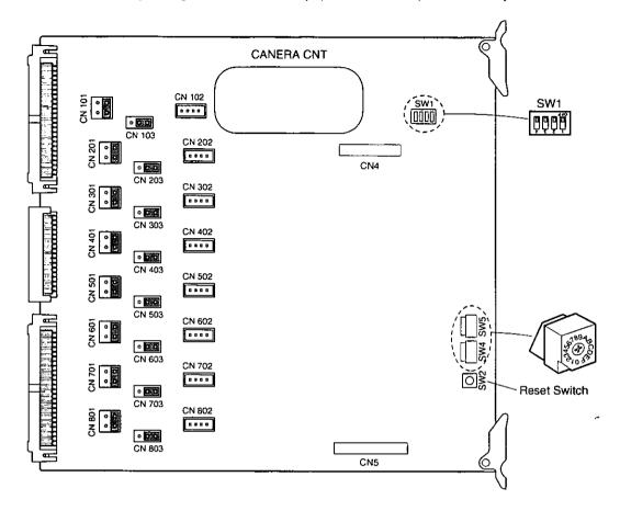
1. Set switches (SW4 and SW5) on the board to designate the camera input board number as shown in the following table. The factory default setting is Board Number 1 (00)
