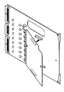
3. Fix both boards with the two supplied screws (M3x6) as shown below.
