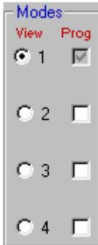
Clicking the **View** option button allows you to view permissions for the mode chosen, and defaults to programming for the same mode. In the case of the graphic to the left, mode 1 is set for viewing, and thereby programming. See Scheduled Modes in the Admin Console manual.
