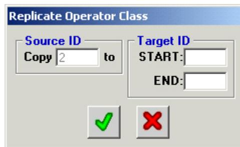
The copy source is the highlighted operator ID from which the subsequent operator classes will be copied.
