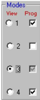
More than one mode can be programmed at the same time by clicking on the **Prog** check boxes of the other mode numbers that you wish to program simultaneously. This will append, or add any permissions that are then changed on the permissions grid, but will not duplicate entire modes or overwrite existing permissions in the other modes.
