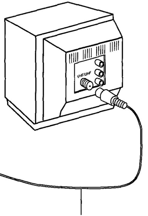
RF Coaxial Cable (VCR-TV Connection Cable) (supplied)
