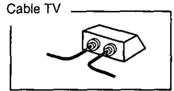
Disconnect the antenna or cable from your TV and connect it to the VCR (IN FROM ANT.)
