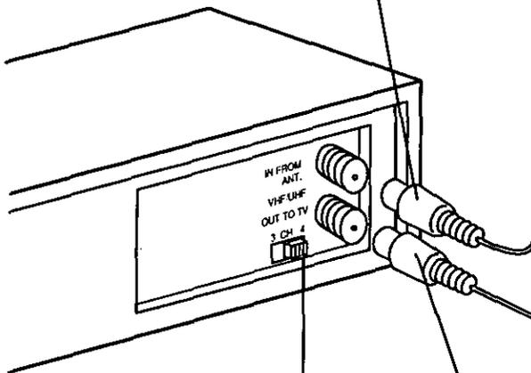
Set the Output Channel of your VCR to channel 3 or 4 (whichever is not being transmitted on by a Local TV broadcast).
