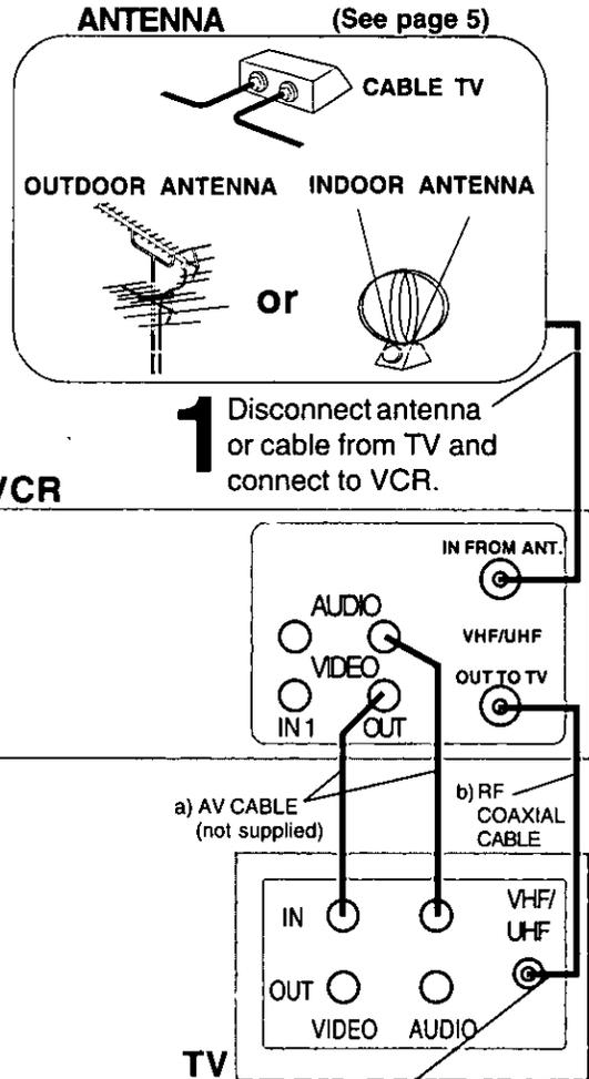
**1** Disconnect antenna or cable from TV and connect to VCR.
