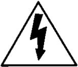
This symbol warns the user that uninsulated voltage within the unit may have sufficient magnitude to cause electric shock. Therefore, it is dangerous to make any kind of contact with any inside part of this unit.
